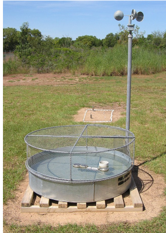
Figure 2.1: Important measurement devices for two fundamental hydrologic variables, which measure the change in depth of liquid water.
