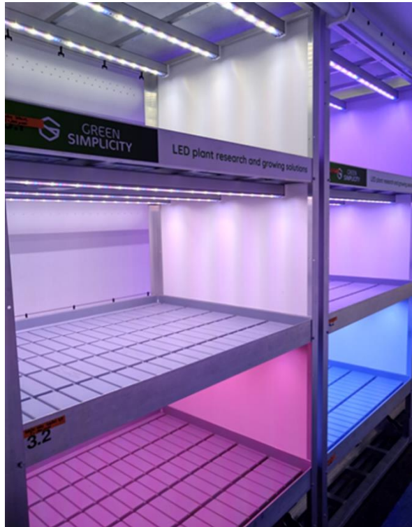
Supplementary Figure 2. Growth chamber (Green Simplicity) used for experimental purposes installed in Hortensia France company. This growth chamber contains several independent LED light modules. Environmental conditions (temperature, relative humidity, CO 2 levels, irrigation) were the same for all modules. Photoperiod, light quality and quantity are controlled independently for each module.
