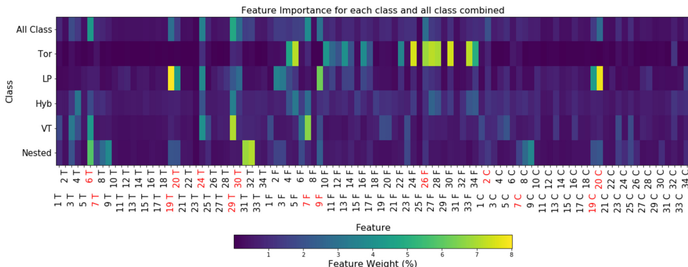
Fig. 6. Weights as percentages for all of the features, for each class, and for all classes combined for the volcanic seismicity detected at La Soufrière de Guadeloupe (January 1, 2013, to December 31, 2018; OVSG-IPGP) determined with the feature importance function in the scikit-learn library. Blue, poor importance in the classification; yellow, important for the classification; red, the 14 most useful features with which the classification is similar to the mean score obtained for the whole feature set.
