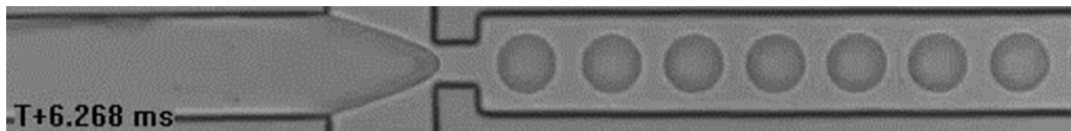
Video 1. Formation of water droplets in a microfluidic chip. See https://vimeo.com/396910891 . By injecting oil and water into different channels of the microfluidic circuit, the experimenter can witness the formation of droplets in real time, on the screen connected to the microscope. In the video, motion is slowed by 200 times.
