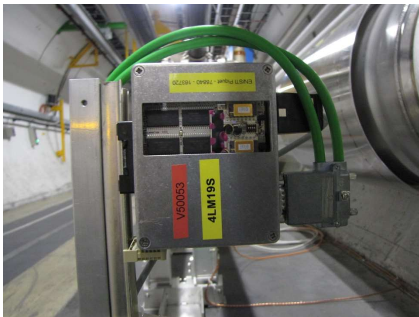
Figure 15 - RADMON system including RadFET for radiation monitoring in the CERN accelerator complex [44]
