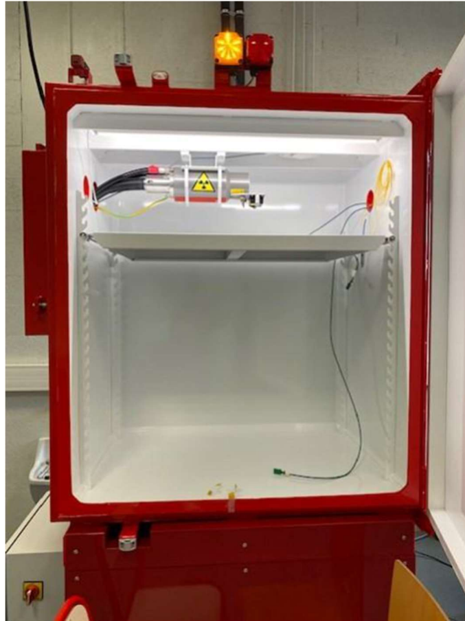
Figure 39 - LABHX X-rays irradiation source located in the Laboratoire Hubert Curien of Saint-Etienne, France.
