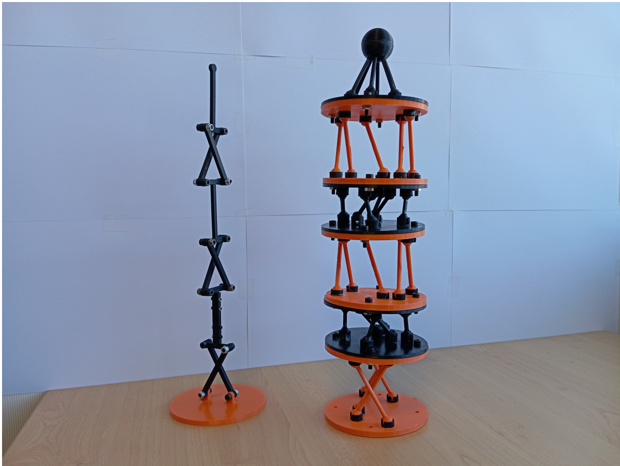
Figure 7.26 – Plastic prototypes of the 3-X spatial manipulator with planar X-joints (left) and modified X-joints (right).
