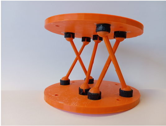
(a) Modified X-joint with five bars
