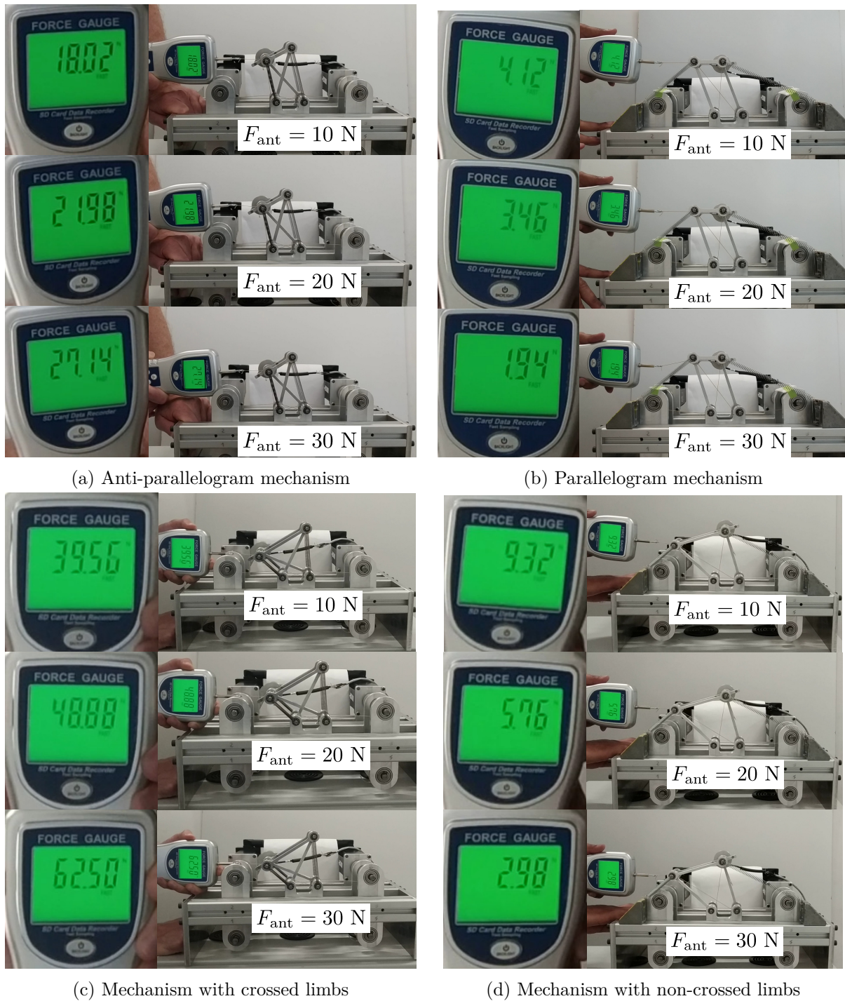
Figure 2.19 – External force required to produce the same displacement in a mechanism for different antagonistic actuation forces F_1 = F_2 = F_{ant} .
