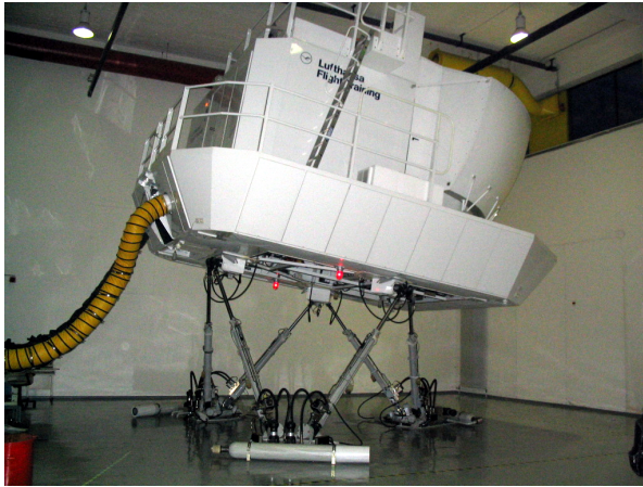
(a) Gough-Stewart platform as flight simulator (Source: [Hex])
