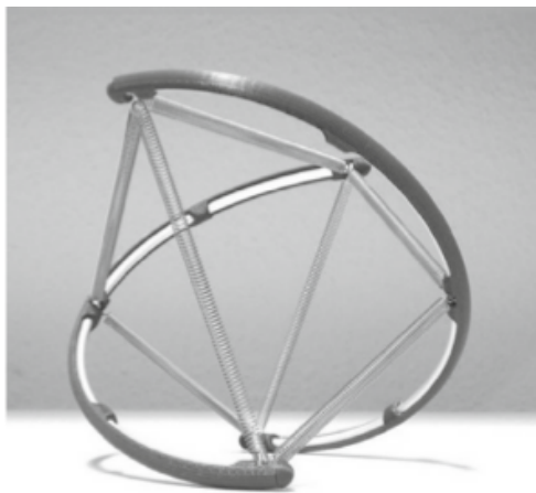
(a) Tensegrity-based spherical mobile robot (Source: [Böh+17])
