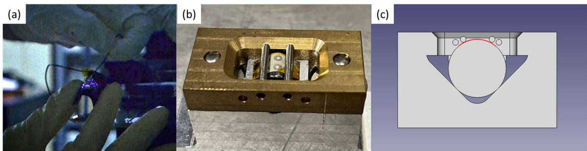
Figure V-19: (a) Flexible device being bent by hand during operation, (b) image of the apparatus for measurements under controlled bending, and (c) scheme of the apparatus presented in (b) with the membrane in red.
