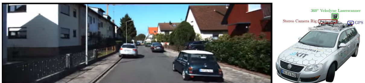
Figure 2.4: Examples of image and capture setup from the dataset Kitti [29]. The vehicle is equipped with GPS, laser and stereo cameras to capture an annotated video flux.
