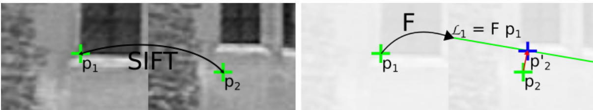
Figure 2.13: From an imperfect match (p_1, p_2) considered inlier by AC-RanSaC, the “perfect match” (p_1, p'_2) is constructed using p'_2 the orthogonal projection of p_2 on the epipolar line \mathcal{L}_1 = F p_1 where F is a realistic fundamental matrix given by AC-RanSaC. This does not guarantee that p'_2 represents the same physical point as p_1 , but that some 3D point at possibly different depth projects exactly at p_1 and p'_2 . Figure originates from [77].
