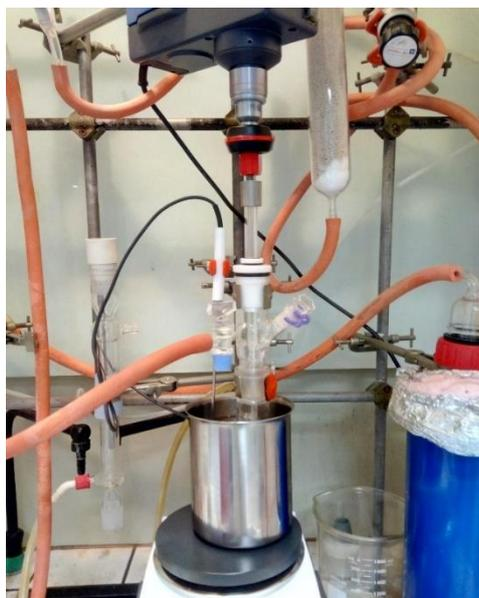
**Figure S12:** Set up for kinetic studies on PUs synthesis from bis-oxamic acids using PIDA-mediated process
