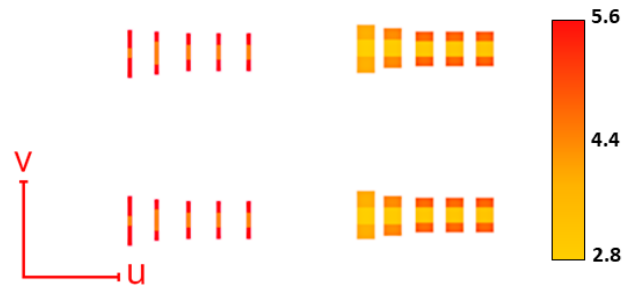
Figure 3.23: GDSII design of antenna after proximity effect correction. The color bar represents the dose factor of the exposure area.
