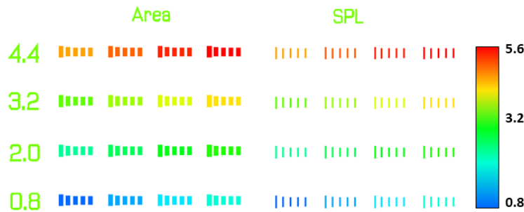
Figure 3.18: Test design of Area and single pixel line pattern. The color bar represents the dose factor of the exposure area.
