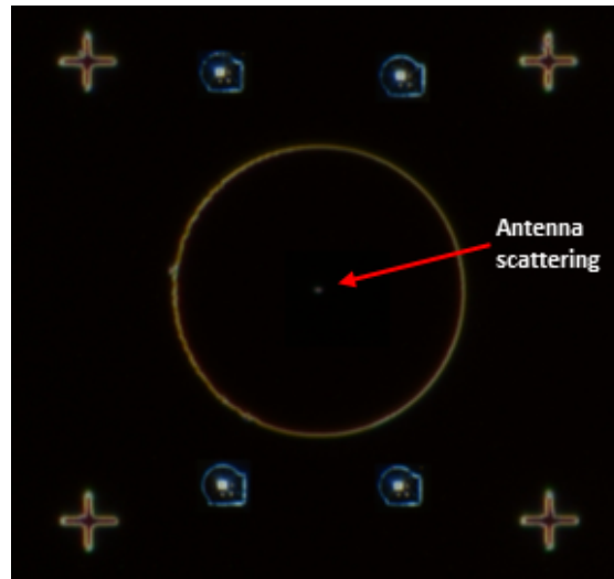
Figure 4.19: Dark field image of Yagi-Uda antenna on TiO 2 microdisk. We observe scattering at the edge of the TiO 2 microdisk and on Yagi-Uda at the center. Cross marks were used for rough alignment and square are PMMA residue after precise alignment. Dots in white squares are precise marks.
