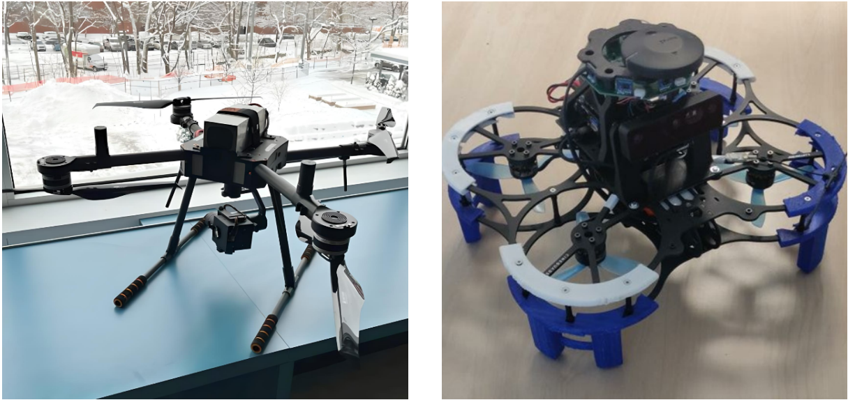
Figure 1.3 – Quadrotor UAVs equipped with an embedded system and various sensors for the BlueSwarm system [23] (left) and the TeamAware project [25] (right).
