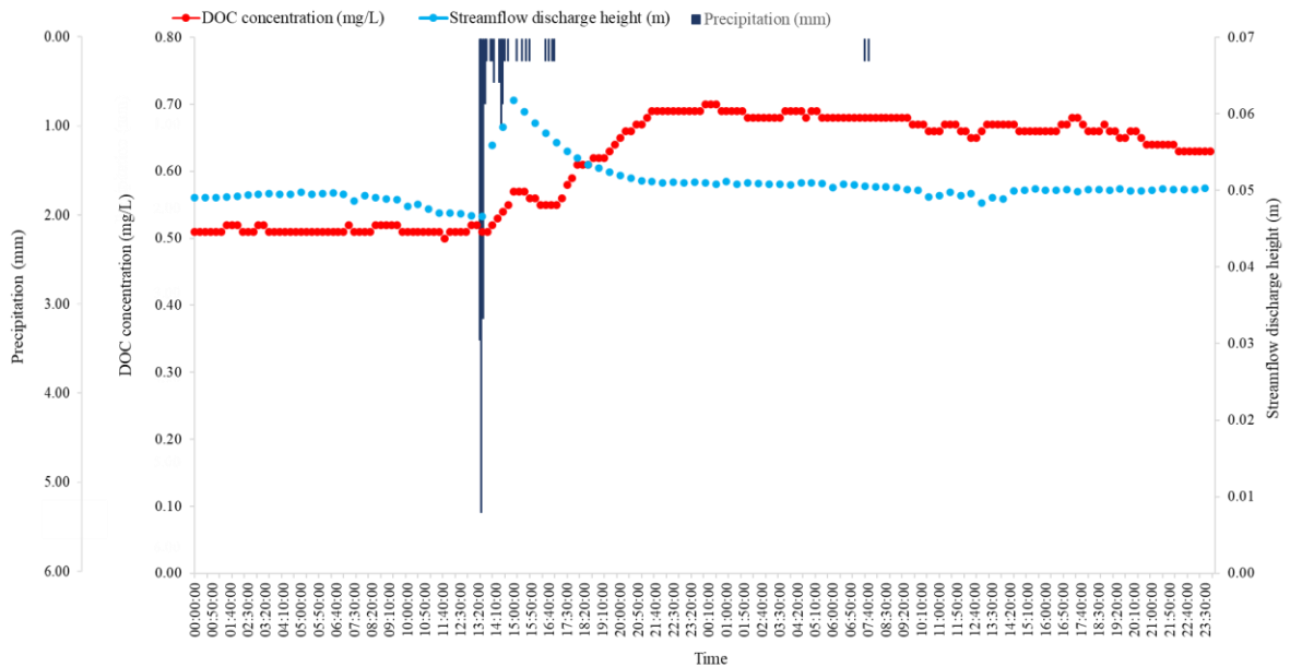
Figure 8.14: Correlations between rainfall, streamflow discharge and DOC probe concentrations during a rainfall event on the 28th of November 2019 for CP-VI and CP-IX
