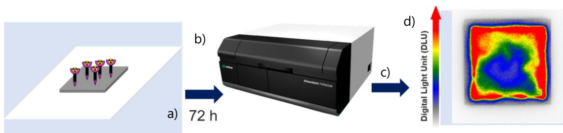
Figure 44: Illustration of the autoradiography: a) exposure of a source (grey) on the imaging plate (white) b) autoradiography imaging system c) reading step in the scanner, d) signal of the source
