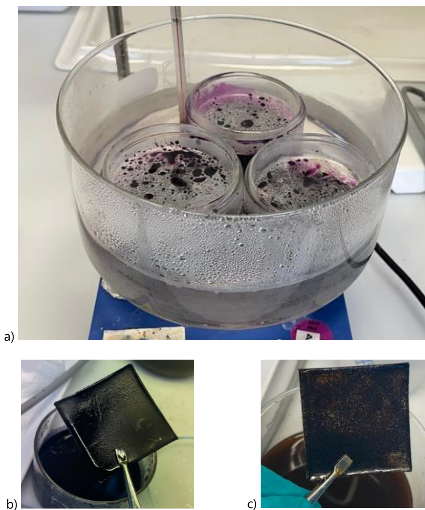
Figure 41: a) Experimental set up for the oxidation of epoxy samples, b) an oxidized sample before washing for 1 h, c) an oxidized sample after washing with acetic acid and DI water
