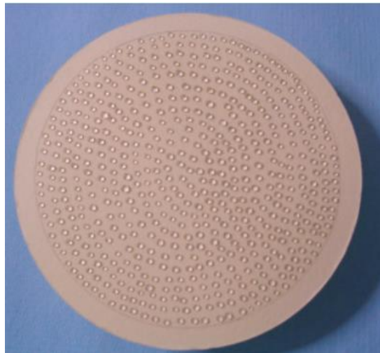
Figure 6: Drop deposition of radioactive solution on a filter paper (Monsanglant-Louvet et al., 2015)
