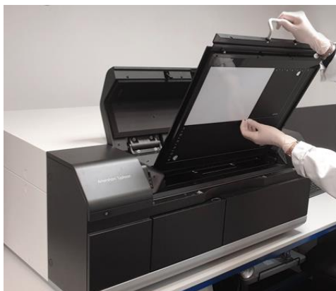
Figure 116: Placing of an autoradiography plate in the device
