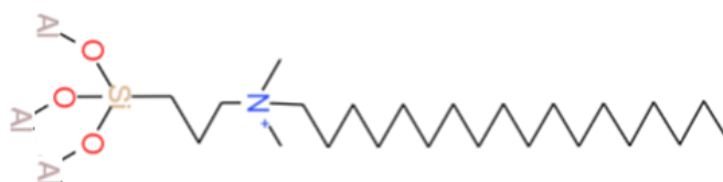
Figure 84: Si-N chemical attaches onto the aluminum surface
