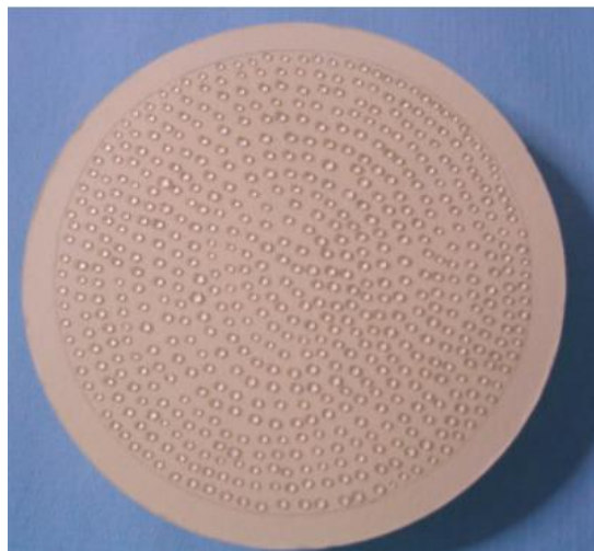
Figure 6: Drop deposition of radioactive solution on a filter paper (Monsanglant-Louvet et al., 2015)
