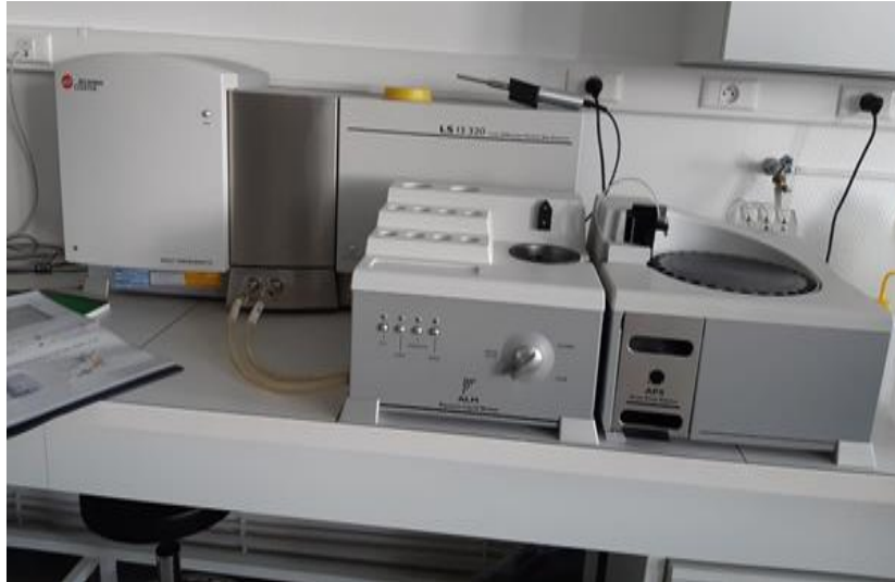
Figure 2. 4. Laser granulometry setup in M2C lab
