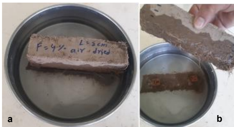
Figure 4. 28. Capillarity water absorption test
