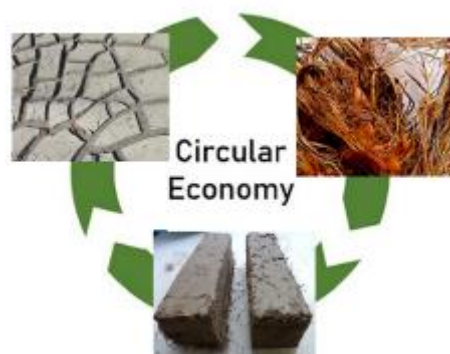
Figure 1. Earth bricks made with sediments and natural fibers.
