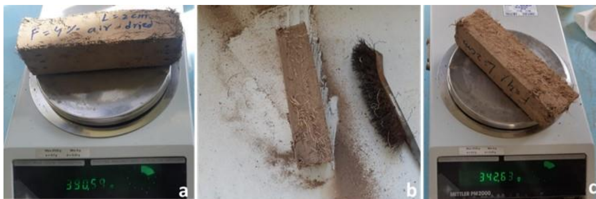
Figure 4. 27. Abrasion testing of earth bricks
