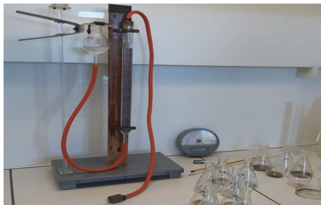
Figure 2. 9. Bernard calcimeter set up in M2C lab
