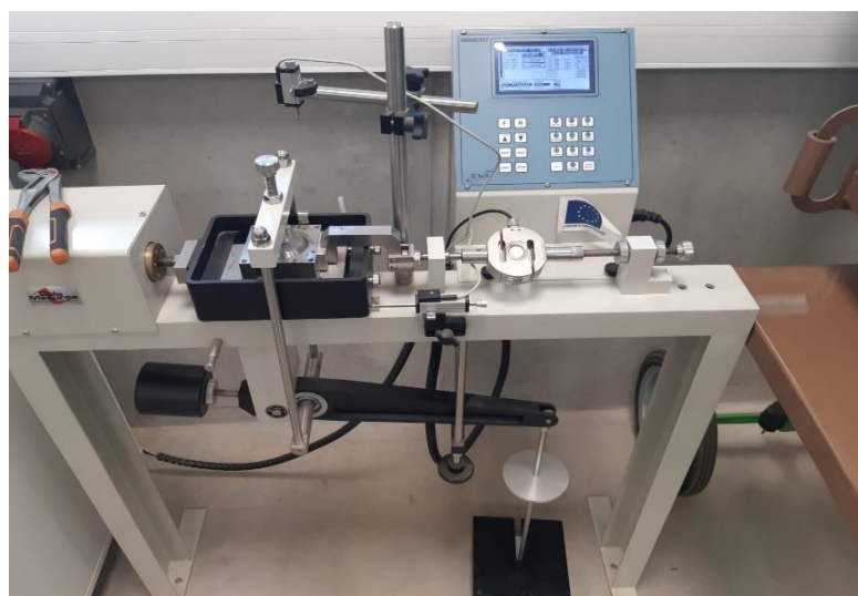
Figure 2. 12. Direct shear test apparatus
