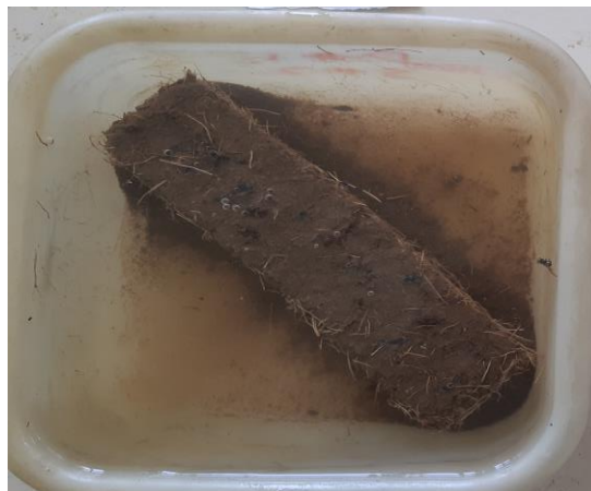
Figure 4. 29. Adobe brick immersion in water
