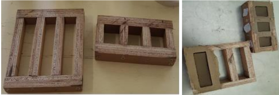
Figure 3. 13. Prismatic and cubic moulds
