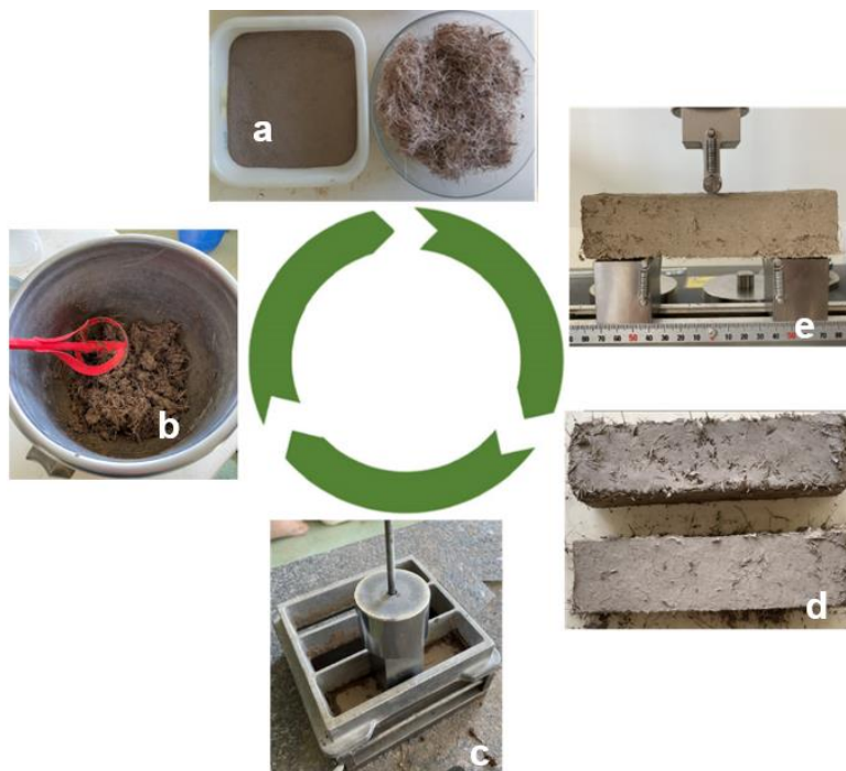
Figure 4. 19. Earth bricks manufacturing process
