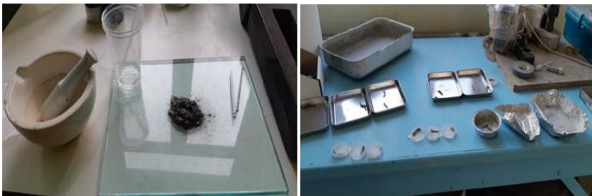
Figure 2. 6. Sediment mixture and rolls to observe plasticity limit
