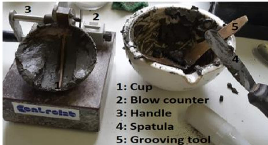
Figure 2. 5. Casagrande apparatus for liquidity test
