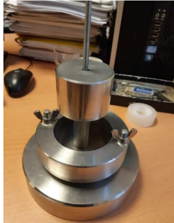
Figure 2. 11. Proctor miniature test apparatus
