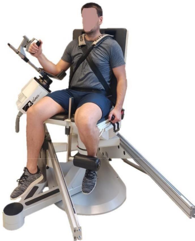
Figure 1 — Setup for isokinetic testing of shoulder internal and external rotators in the seated position.
