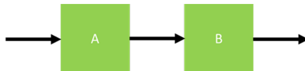
Figure 3.12 – RBD representation of elements A and B in series
