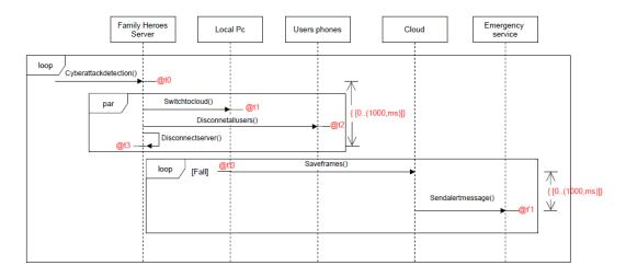
Figure 3.10: UML sequence diagram in fall and cyber-attack scenario.
