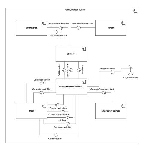
Figure 3.4: UML components diagram of Family Heroes system.
