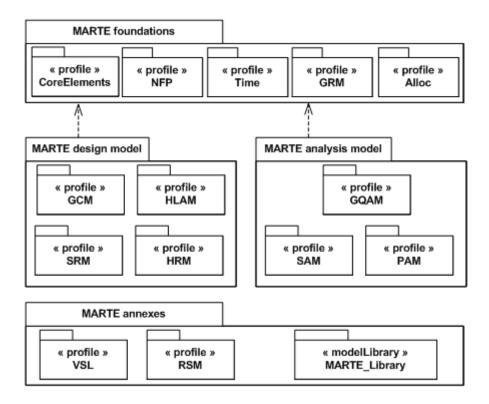
Figure 2.2: Architecture of the UML MARTE profile [57]
