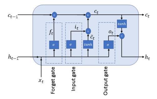
Figure 4.3: LSTM unit architecture.
