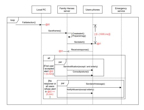
Figure 3.6: UML sequence diagram with time constraints of the Family Heroes system.
