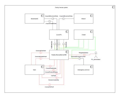
Figure 3.9: UML components diagram of the alternative solution.
