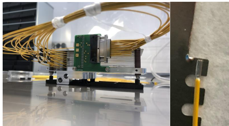
Figure 3.7: Left panel: Photograph of the energy analyser assembled with the voltage divider PCB mounted on its side. The photography also shows how the potentials are brought to the EA’s guard plates. Right panel: photograph of the electrical soldering using crimped Ni tubes.
