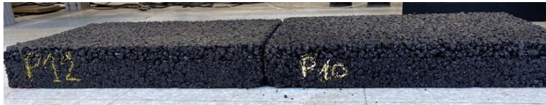
(b) Vertical crack within a surface layer simulated as horizontal discontinuity between two bilayer HMAs
