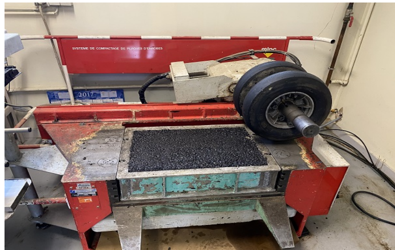
(a) Devices for compacting asphalt plates
