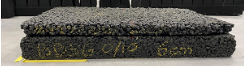
(a) Horizontal detachment inside a surface layer simulated with VTBC placed on STBC without a tack coat
