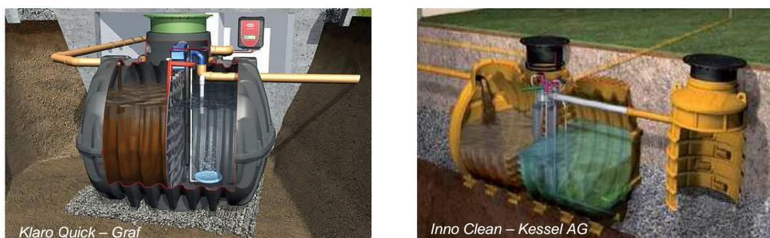
Figure I- 11. Exemples de microstations SBR (Graf, 2013 ; Kessel, 2013 )
