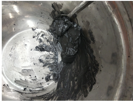
(c) Paste of CM2 asteroid simulant made with the addition of water to the mix
