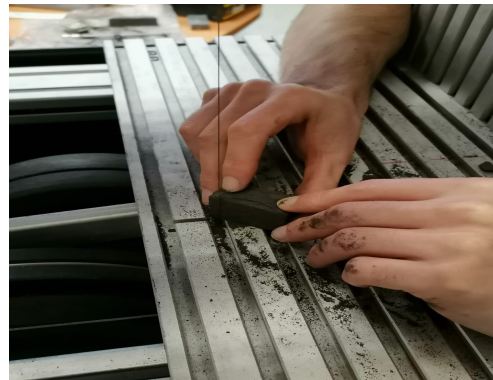
(d) Machining of a sample for tensile strength characterization (step 4) : Shaping of the sample by line tracking with a wire saw
