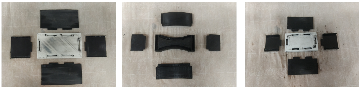
(a) Rectangular sample (40 x 40 x 80 mm) (b) Tensile strength sample (c) Rectangular sample (20 x 20 x 40 mm)
