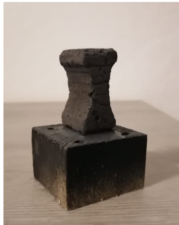
Figure 2.16: Tensile test sample glued on a piece of wood
