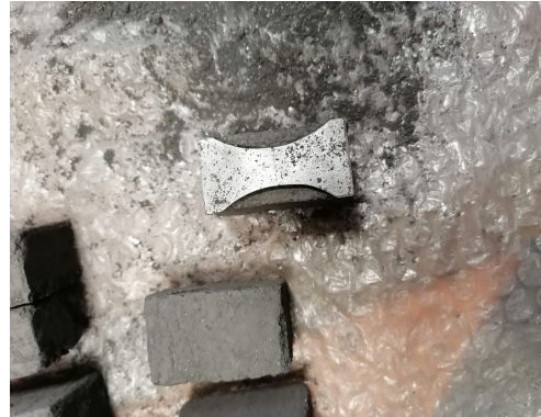
(b) Machining of a sample for tensile strength characterization (step 2) : Use of an aluminum pattern
