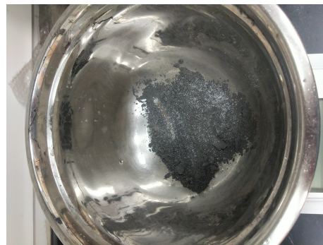
(b) Powder of CM2 asteroid simulant mixed with glass beads
