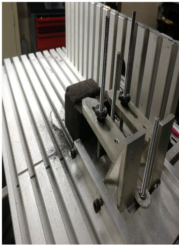
(a) Cutting 20 mm thick slices with a wire saw
