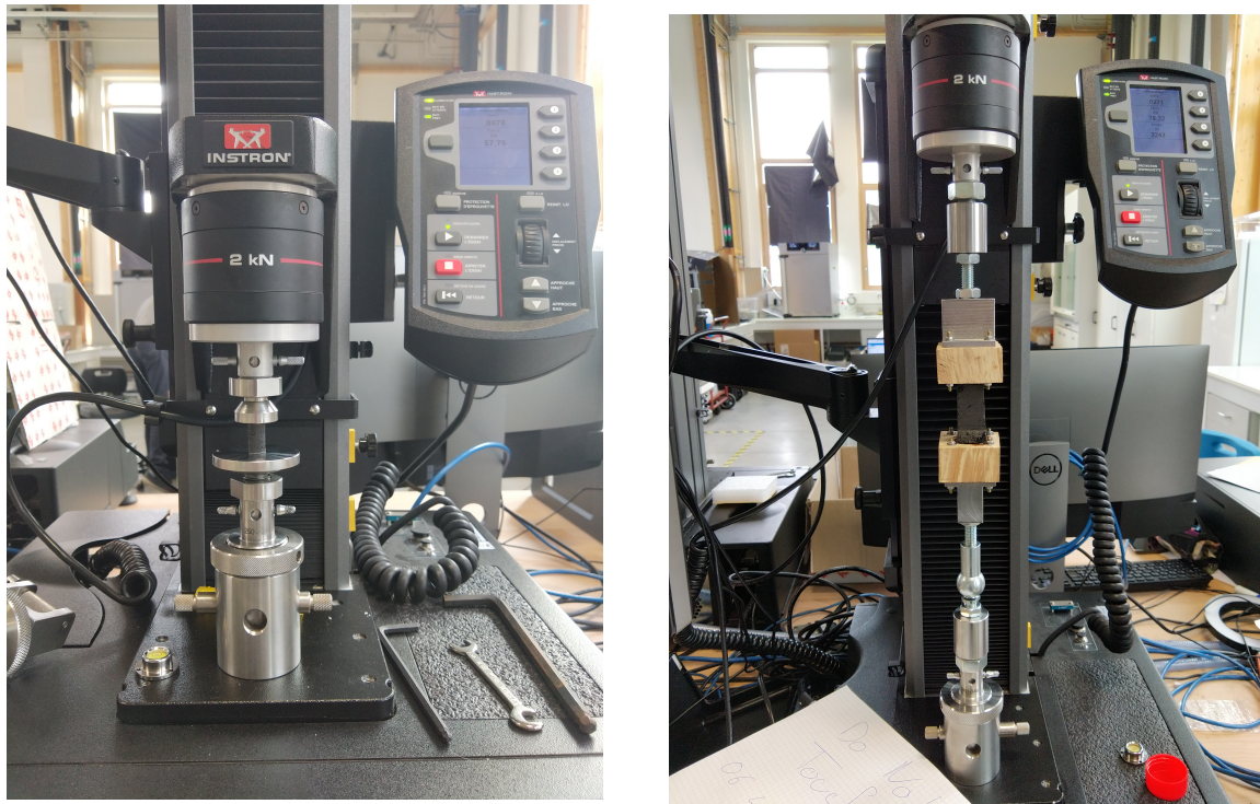
(a) Compression Set-up No. 1 : Identical to the experiment carried out by Avdellidou et al. (2019b) (b) Compression Set-up No. 2 : Glued sample
