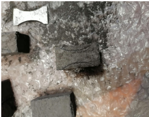
(c) Machining of a sample for tensile strength characterization (step 3) : Engraving the shape of the sample on the material
