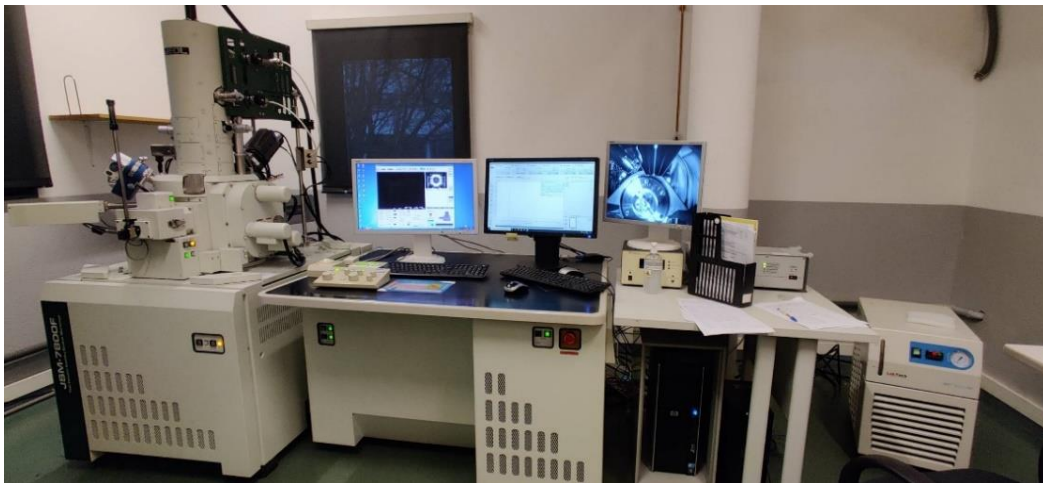
Figure 2.7: The Scanning Electron Microscope (SEM, JEOL JSM-7800F) equipped with an Energy Dispersive X-ray Spectroscopy (EDS) [1]
