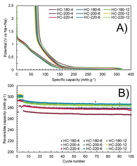
**Figure 21: A)** First cycle discharge-charge and **B)** cycling behaviour of the hard carbons from the hydrochars at the different conditions. The 5 first cycles are performed at C/10 then at 1C until the  $100^{th}$  cycle ( $C = 372 \text{ mA.g}^{-1}$ ).
