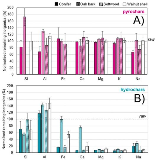
**Figure 74:** Normalised remaining inorganics in % of the major elements in **A)** the pyrochar and **B)** the hydrochar for the 4 biomasses. They were calculated according to equation **(9)**. Standard deviations are experimentals.
