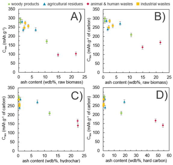
**Figure 51: A)**  $C_{rev}$  per gram of material depending on the raw biomass ash content, and  $C_{rev}$  per gram of carbon depending on the ash content in **B)** the raw biomass, **C)** the hydrochar and **D)** the hard carbon.
