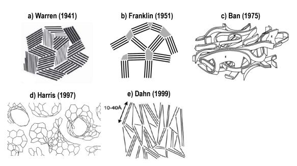
**Figure 5:** Evolution of hard carbon structure representation, adapted from [21] and [27] from the original works of [23]–[26], [28].
