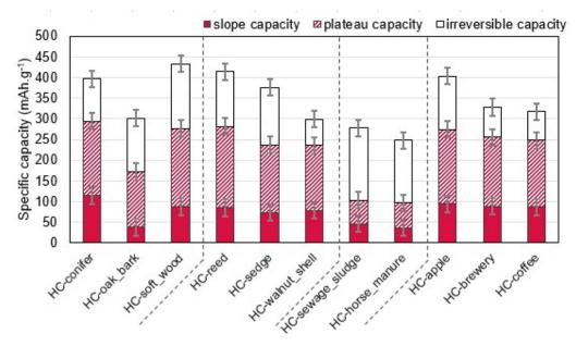
**Figure 54:** Slope and plateau capacities of the charge and irreversible capacity at the discharge of the first cycle. Uncertainties are from the method used.
