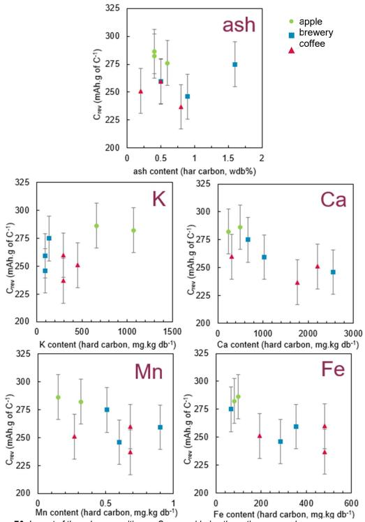
**Figure 70:** Impact of the ash composition on C<sub>rev</sub>, considering the active mass only.
