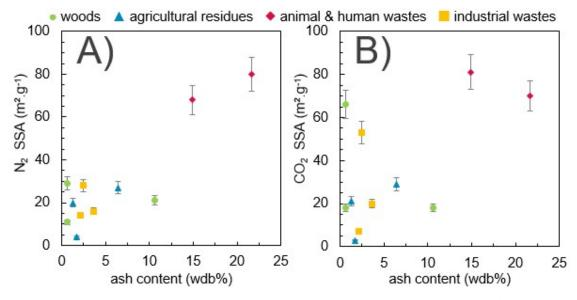
**Figure 44:** Influence of the raw biomass ash content on **A)** the  $N_2$  SSA and **B)** the  $CO_2$  SSA of the hard carbon. Uncertainties are from the method used.
