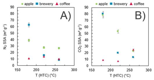
**Figure 67: A)** N<sub>2</sub> and **B)** CO<sub>2</sub> SSA of the hard carbon depending on the HTC temperature.
