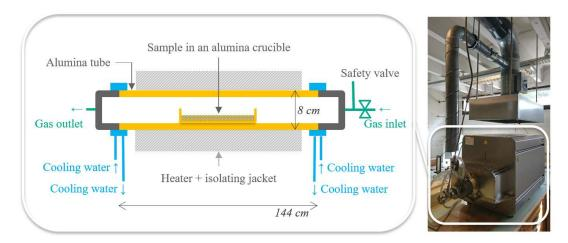
Figure 15: High temperature pyrolysis oven schematic and picture
