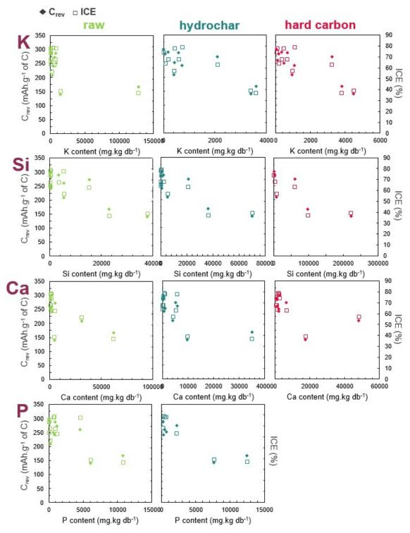
**Figure 52:** Influence of the K, Si, Ca and P contents of the raw material (green), hydrochar (blue) and hard carbon (red) on the reversible capacity  $C_{rev}$  ( $\spadesuit$ ) and ICE ( $\square$ ). The axis for  $C_{rev}$  is on the left, while the secondary axix for ICE is on the right. P content in tha hard carbon was not measured.
