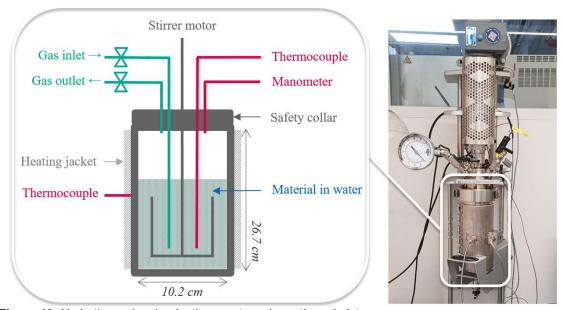
Figure 13: Hydrothermal carbonisation reactor schematic and picture
