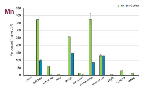
**Figure 35:** Balance of the Mn between the raw material (in green) and the hydrochar (in blue). To compare de value, hydrochar contents have been converted in mg.kg raw db<sup>-1</sup> according to equation **(10)**.
