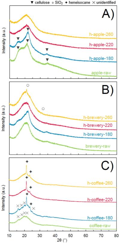
**Figure 63:** XRD patterns of materials from **A)** apple pomace, **B)** brewery waste and **C)** spent coffee grounds. Peaks are identified with symbols as:  $\blacktriangledown$  Cellulose-Iβ ( $C_6H_{10}O_5$ )<sub>n</sub> (PDF 00-060-1502),  $\circ$  crystobalite beta. Syn SiO<sub>2</sub>. (PDF 01-077-8630),  $\blacklozenge$  n-heneicosane  $C_{21}H_{44}$  (PDF 00-031-1705) and  $\times$  unidentified.
