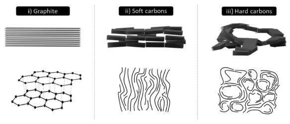
Figure 4: Organisation of graphene layers in carbon materials [20].
