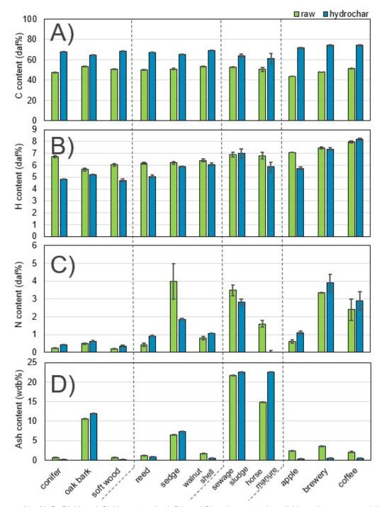
**Figure 27: A)** C, **B)** H and **C)** N content in daf% and **D)** ash content in wdb% on the raw materials (in green) and hydrochars (in blue). Uncertainties are the standard deviations between the replicates for C, H and N contents, and the method deviation for the ash.
