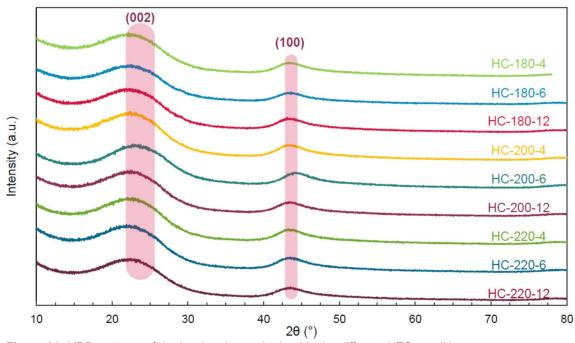
Figure 20: XRD patterns of the hard carbons obtained in the different HTC conditions.
