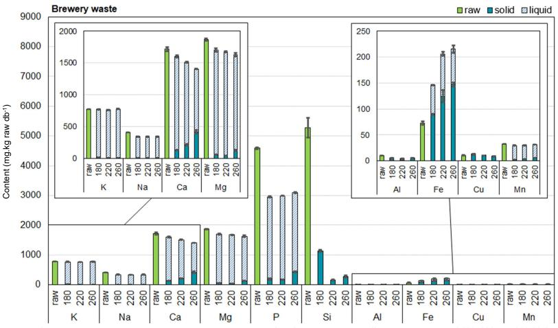
**Figure 61:** Balance of the inorganics between the raw material and the hydrochar (solid) and liquid at the different temperatures of 180, 220 and 260 °C from brewery waste. The different elements were represented on different scale, depending on the content. The values were converted on mg of element per kg of raw biomass according to equations (10) and (11) for solids and liquids respectively in order to compare them together. Standard deviation are experimental between the replicates.
