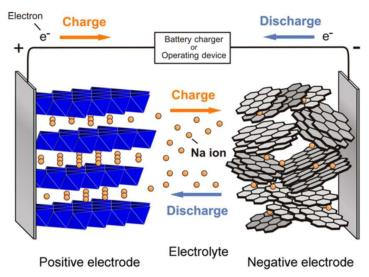
Figure 1: Sodium-ion battery principle, from [14].
