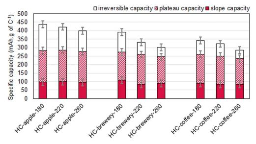
**Figure 71:** Slope and plateau capacities of the charge and irreversible capacity at the discharge of the first cycle. Uncertainties are from the method used.
