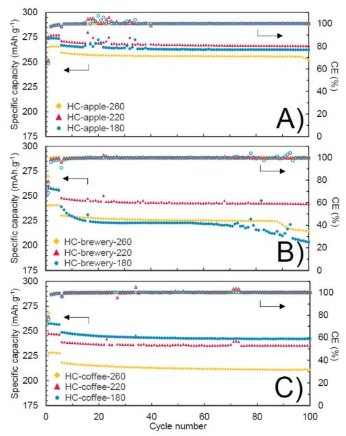
**Figure 72:** Cycling behaviour of **A)** apple-, **B)** brewery- and **C)** coffee-based material from the different hydrochar obtained at 180 °C (blue), 220 °C (red) and 260 °C (yellow). The 5 first cycles are performed at C/10 then at 1C until the  $100^{th}$  cycle (C = 372 mAh). The plots are from 1 experimental cell, reproducible between replicates.
