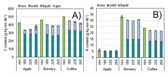
**Figure 59: A)** Carbon and **B)** Nitrogen balances at the different temperatures for the solid, liquid and gas fractions. The values were converted to g of element per kg of raw biomass dry basis. Carbon in the liquid is calculated from the total organic carbon of the total C. Carbon in the gas phase is deduced from the produced CO<sub>2</sub>. Nitrogen in the liquid is deduced from the measured total nitrogen. Standard deviations are experimental between the replicates.
