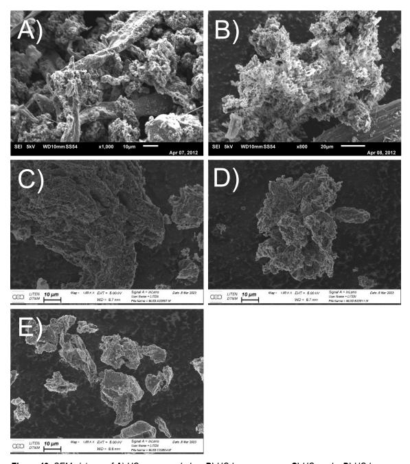
**Figure 42:** SEM pictures of **A**) HC-sewage\_sludge, **B**) HC-horse\_manure, **C**) HC-apple, **D**) HC-brewery, and **E**) HC-coffee.
