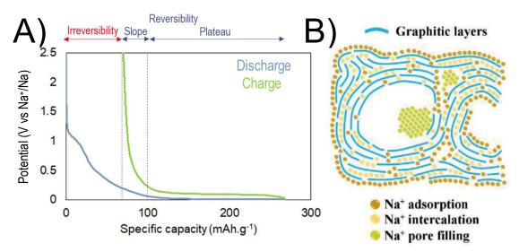
**Figure 8: A)** Typical hard carbon first cycle reduction – oxidation pattern and **B)** Schematic illustrations of Na<sup>+</sup> storage in hard carbon [29].
