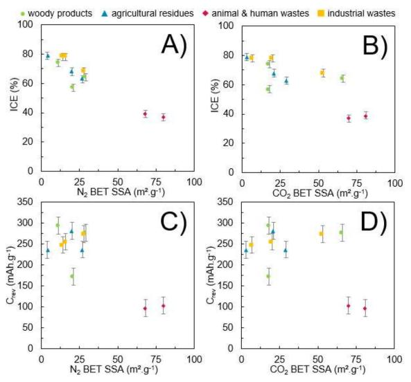
**Figure 50:** ICE depending on the **A)**  $N_2$  BET SSA and the **B)** CO<sub>2</sub> BET SSA of the hard carbon, and  $C_{rev}$  depending on the **C)**  $N_2$  BET SSA and the **D)** CO<sub>2</sub> BET SSA of the hard carbon. Uncertainties are from the method used.
