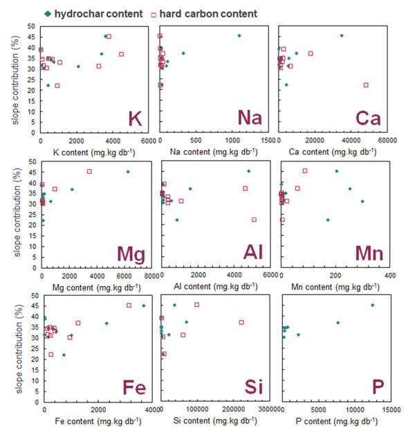
**Figure 57:** Contribution of the slope in  $C_{rev}$  depending of the inorganic contents in the hydrochars ( $\diamond$ ) and hard carbons ( $\Box$ ). P was not measured in the hard carbons.
