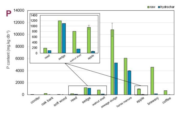
**Figure 36:** Balance of the P between the raw material (in green) and the hydrochar (in blue). To compare de value, hydrochar contents have been converted in mg.kg raw db<sup>-1</sup> according to equation **(10)**.
