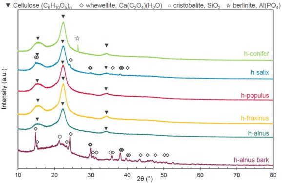
**Figure 19**: XRD patterns of the hydrochars obtained from the six driftwood. Peaks are identified as: ▼ Cellulose-I $\beta$  ( $C_6H_{10}O_5$ )<sub>n</sub> (PDF 00-060-1502),  $\diamondsuit$  Calcium oxalate hydrate, whewellite, Ca( $C_2O_4$ )( $H_2O$ ) (PDF 04-025-6897),  $\diamondsuit$  Silicon oxide, cristobalite. high. syn SiO<sub>2</sub> (PDF 04-008-7643) and  $\Leftrightarrow$  Aluminium phosphate, Berlinite, syn Al(PO<sub>4</sub>) (PDF 04-009-5761).
