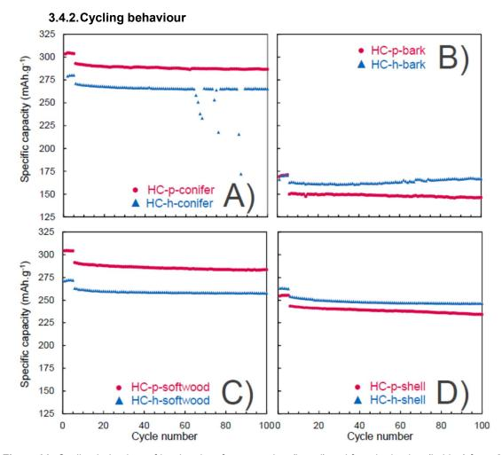
**Figure 83:** Cycling behaviour of hard carbon from pyrochar (in red) and from hydrochar (in blue) from **A)** conifer (wet), **B)** oak bark, **C)** softwood, **D)** walnut shell. The 5 first cycles are performed at C/10 then at 1C until the  $100^{th}$  cycle (C = 372 mA.g<sup>-1</sup>).
