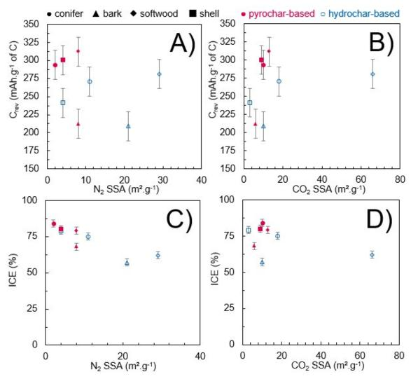
**Figure 81:** Influence of **A)**  $N_2$  BET SSA, **B)** CO<sub>2</sub> BET SSA on the  $C_{rev}$ , and **C)**  $N_2$  BET SSA, **D)** CO<sub>2</sub> BET SSA on the ICE. The pyrochar-based materials are represented in full red symbols, while hydrochars based are empty blue.
