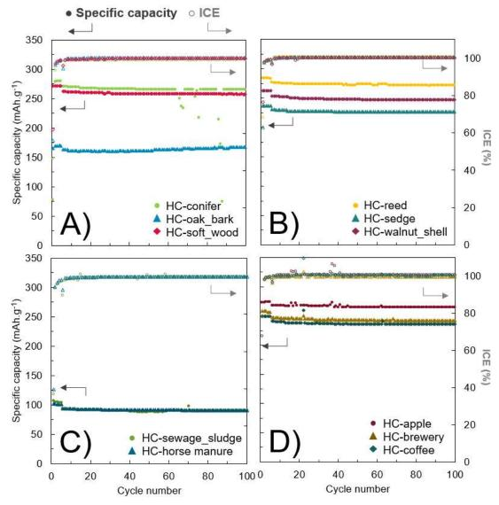
**Figure 49:** Cycling behaviour of **A)** woody product, **B)** herbaceous and agricultural residue, **C)** animal and human wastes and **D)** industrial biomass wastes. The 5 first cycles are performed at C/10 then at 1C until the  $100^{th}$  cycle (C = 372 mA.g<sup>-1</sup>).
