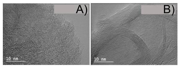
**Figure 6:** TEM picture of hard carbon from washed **A)** asparagus peel and **B)** grape waste synthetised on the same conditions, adapted from [30]. The image on the left shows small-range organisation, while bigger organised areas, made of more and longer sheets on the right.
