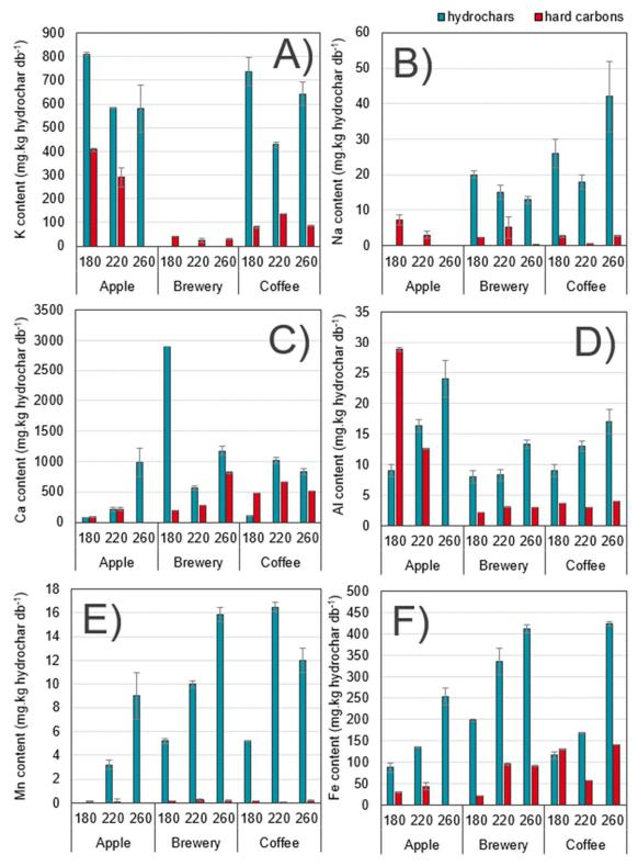
**Figure 64:** Remaining **A)** K, **B)** Na, **C)** Ca, **D)** Al, **E)** Mn, **F)** Fe contents in the hydrochar (blue) and the hard carbon (red) from all agro-food feedstock. The values were converted on mg of element per kg of hydrochar similarly to equation (10) in order to compare them together. Standard deviations are experimental between the replicates.
