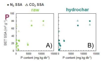
**Figure 47:** Influence of the P content of **A)** the raw material (green) and **B)** hydrochar (blue) on the hard carbon  $N_2$  ( $\bullet$ ) and  $CO_2$  ( $\triangle$ ) SSA.
