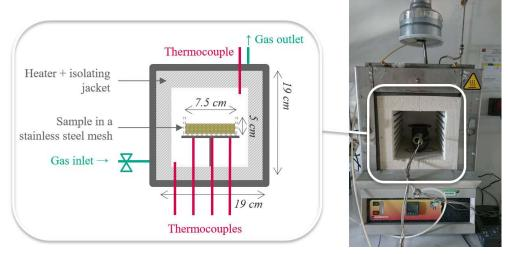
Figure 14: Low temperature pyrolysis oven schematic and picture
