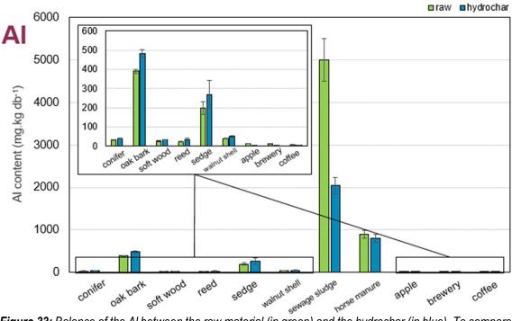
**Figure 33:** Balance of the Al between the raw material (in green) and the hydrochar (in blue). To compare de value, hydrochar contents have been converted in mg.kg raw db<sup>-1</sup> according to equation **(10)**.
