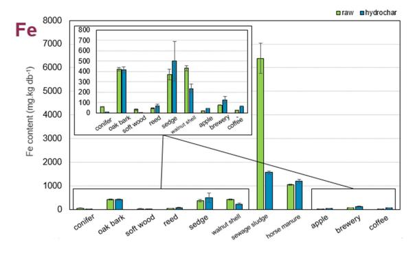
**Figure 34:** Balance of the Fe between the raw material (in green) and the hydrochar (in blue). To compare de value, hydrochar contents have been converted in mg.kg raw db<sup>-1</sup> according to equation **(10)**.
