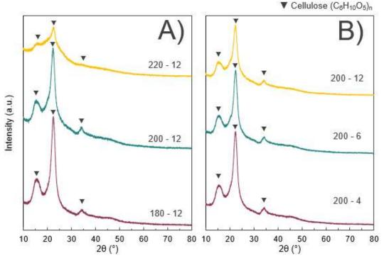
**Figure 18:** XRD patterns of the hydrochar from alnus **A)** at 220, 200 and 180 °C for 12 h and **B)** at 200 °C for 4, 6 and 12 h. Peaks are identified with symbols as:  $\blacktriangledown$  Cellulose-Iβ (C<sub>6</sub>H<sub>10</sub>O<sub>5</sub>)<sub>n</sub> (PDF 00-060-1502).
