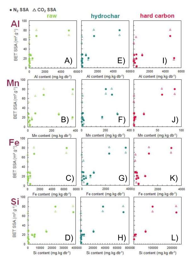
**Figure 46:** Influence of the Al, Mn, Fe and Si contents of **A-D**) the raw material (green), **E-H**) hydrochar (blue) and **I-L**) hard carbon (red) on the hard carbon  $N_2(\bullet)$  and  $CO_2(\triangle)$  BET SSA.
