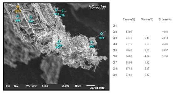
Figure 43: SEM-EDS of HC-sedge on the SiC whiskers.
