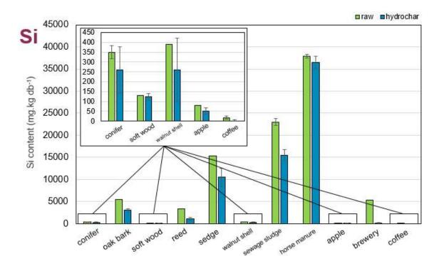
**Figure 37:** Balance of the Si between the raw material (in green) and the hydrochar (in blue). To compare de value, hydrochar contents have been converted in mg.kg raw db<sup>-1</sup> according to equation **(10)**.
