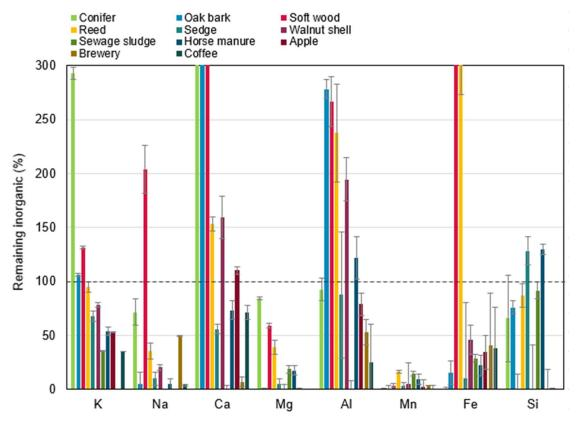
**Figure 39:** Balance of the inorganics that remain in the hard carbon after reaction in %. Values are calculated similarly to equation (9). The lack of histogram bars comes from the hydrochar content that were below limit of detection. Uncertainties are experimental standard deviations.
