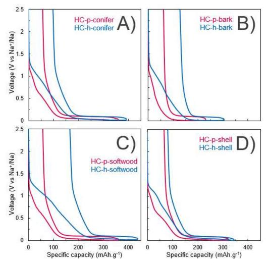
**Figure 80:** First reduction-oxidation profile of hard carbon from pyrochar (in red) and from hydrochar (in blue) from **A)** conifer (wet), **B)** oak bark, **C)** softwood, **D)** walnut shell at C/10 (C = 372 mA. $g^{-1}$ ).
