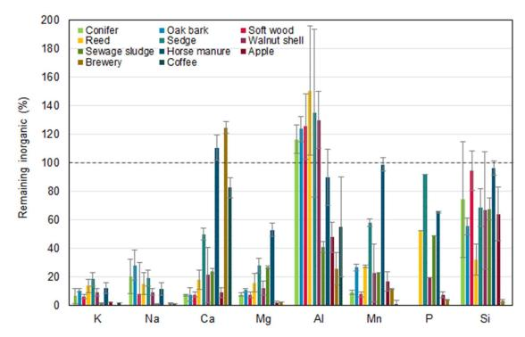
**Figure 28:** Balance of the inorganics that remain in the char after reaction in %. The lack of histogram bars comes from the hydrochar content that were below limit of detection. Uncertainties are experimental standard deviations.
