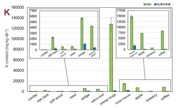
**Figure 29:** Balance of the K between the raw material (in green) and the hydrochar (in blue). To compare de value, hydrochar contents have been converted in mg.kg raw db<sup>-1</sup> according to equation **(10)**.
