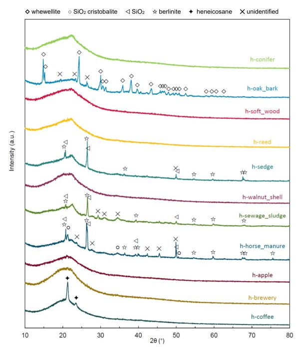
**Figure 38:** XRD patterns of the hydrochars. Peaks are identified with symbols as: ♦ whewellite. syn  $C_2CaO_4$ .H2O (PDF 00-020-0231), ○  $SiO_2$  silicon oxide. crystobalite beta. Syn (PDF 01-077-8630),  $\triangleleft$  Silicon oxide quartz. low  $SiO_2$  (PFD 00-005-0490),  $\nleftrightarrow$  berlinite, syn AlPO<sub>4</sub> (PDF 04-009-5761),  $\spadesuit$  n-heneicosane  $C_{21}H_{44}$  (PDF 00-031-1705), and  $\times$  unidentified.
