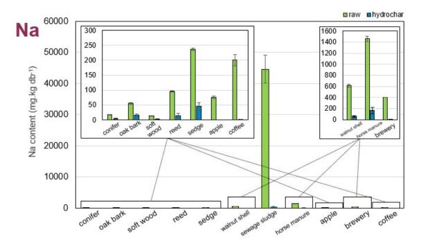
**Figure 30:** Balance of the Na between the raw material (in green) and the hydrochar (in blue). To compare de value, hydrochar contents have been converted in mg.kg raw db<sup>-1</sup> according to equation **(10)**.
