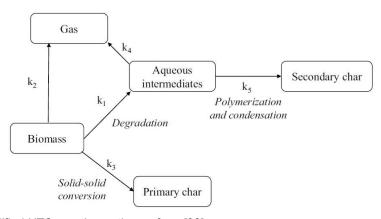
Figure 12: Simplified HTC reaction pathway, from [98]
