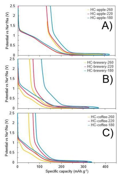
**Figure 68:** First reduction-oxidation profile of **A)** apple-, **B)** brewery- and **C)** coffee-based hard carbon from the hydrochar obtained at 180 °C (blue), 220 °C (red) and 260 °C (yellow) at 37.2 mA.g<sup>-1</sup>. The plots are from 1 experimental cell, reproducible between replicates.
