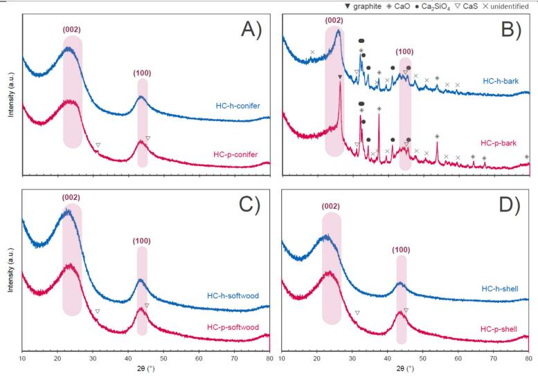
**Figure 76:** XRD patterns of the pyrochar-based (in blue) and hydrochar-based (in pink) hard carbons from **A)** conifer (wet), **B)** oak bark, **C)** conifer (dry) and **D)** walnut shell. Peaks are identified as  $\blacktriangledown$  C, Graphite (PDF 00-001-0640),  $\bullet$  Ca<sub>2</sub>SiO<sub>4</sub>, Larnite (PDF 00-033-0302) and  $\diamondsuit$  CaO, Lime (PDF 00-037-1497),  $\triangledown$  CaS Calcium sulfade Oldhamite, syn (PDF 04-004-3787), and × unidentified.
