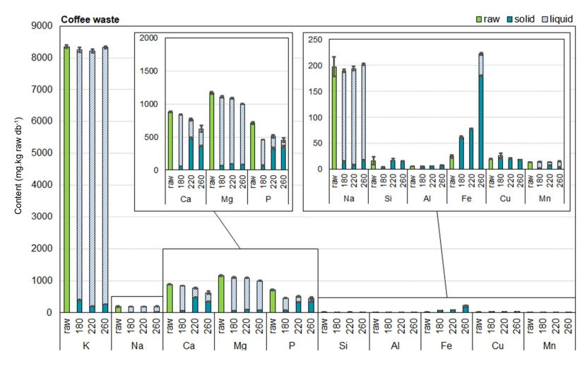
**Figure 62:** Balance of the inorganics between the raw material and the hydrochar (solid) and liquid at the different temperatures of 180, 220 and 260 °C from coffee waste. The different elements were represented on different scale, depending on the content. The values were converted on mg of element per kg of raw biomass according to equations (10) and (11) for solids and liquids respectively in order to compare them together. Standard deviation are experimental between the replicates.
