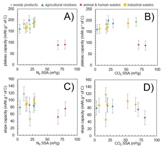
**Figure 55: A)** Plateau capacity depending on the **A)**  $N_2$  SSA and the **B)** CO<sub>2</sub> SSA of the hard carbon, and slope capacity depending on the **C)**  $N_2$  SSA and the **D)** CO<sub>2</sub> SSA of the hard carbon. Uncertainties are from the method used.
