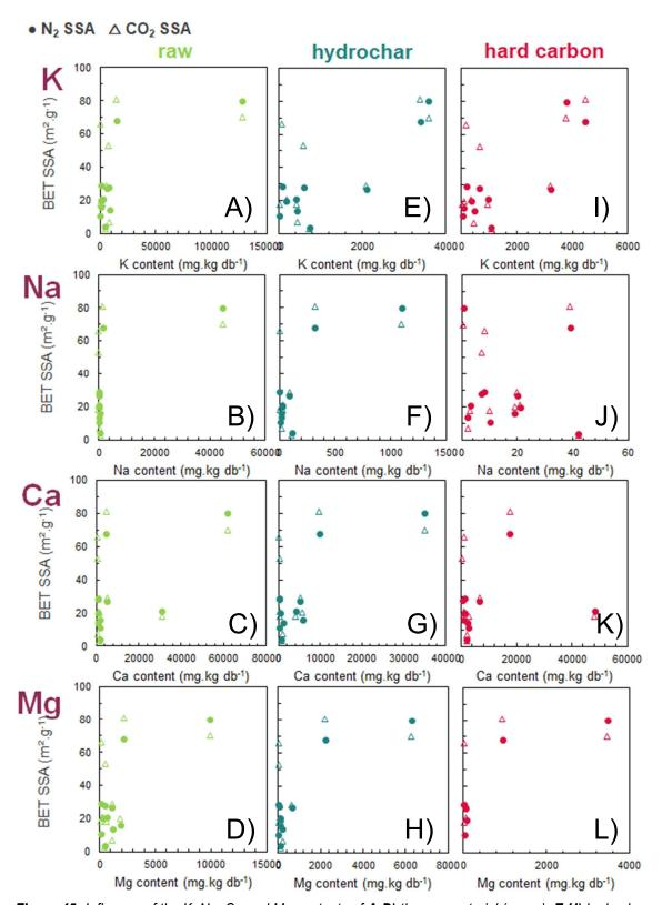
**Figure 45:** Influence of the K, Na, Ca and Mg contents of **A-D)** the raw material (green), **E-H)** hydrochar (blue) and **I-L)** hard carbon (red) on the hard carbon  $N_2$  ( $\bullet$ ) and  $CO_2$  ( $\triangle$ ) SSA.
