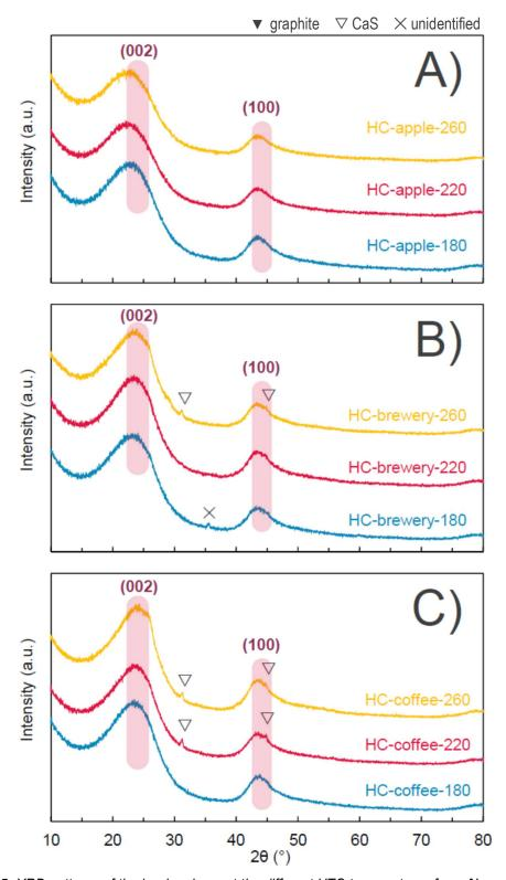
**Figure 65:** XRD patterns of the hard carbons at the different HTC temperatures from **A)** apple pomace, **B)** brewery waste and **C)** spent coffee ground. Peaks are identified with symbols as:  $\nabla$  Calcium sulfide Oldhamite. syn CaS (PDF 04-004-3787), and  $\times$  unidentified.
