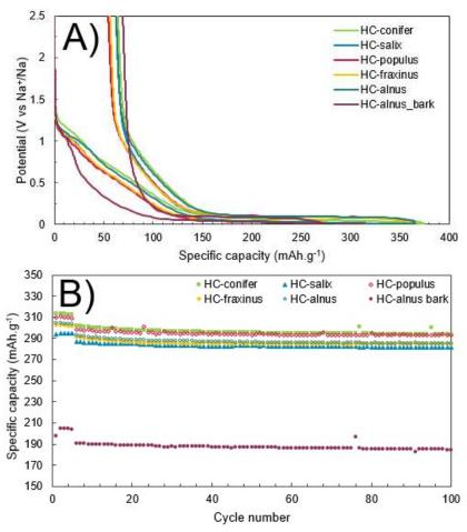
**Figure 24: A)** First cycle discharge-charge and **B)** cycling behaviour of the hard carbons from the six genera. The 5 first cycles are performed at C/10 then at 1C until the  $100^{th}$  cycle (C = 372 mA. $g^{-1}$ ).
