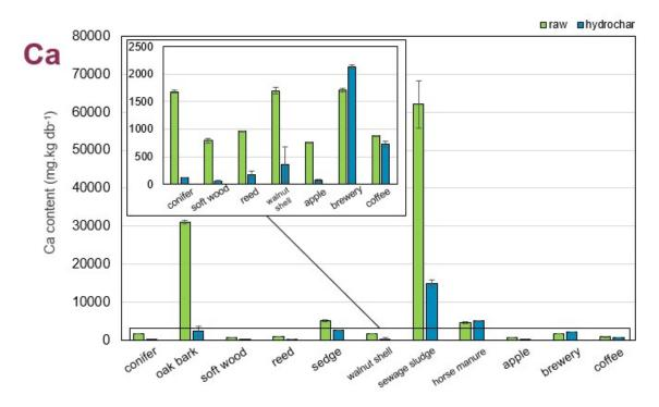
**Figure 31:** Balance of the Ca between the raw material (in green) and the hydrochar (in blue). To compare de value, hydrochar contents have been converted in mg.kg raw db<sup>-1</sup> according to equation **(10)**.
