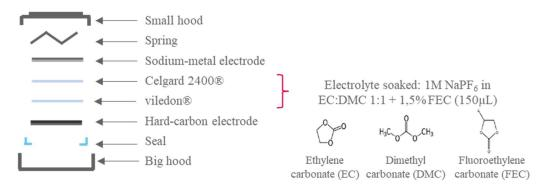
Figure 16: Half-cell assembly.
