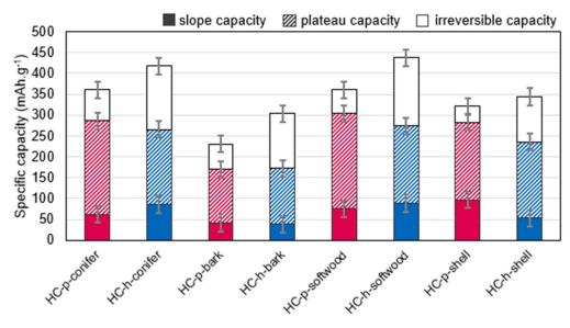
**Figure 82:** Slope, plateau and irreversible capacity distribution of the first cycle at C/10 ( $C = 372 \text{ mA.g}^{-1}$ ).
