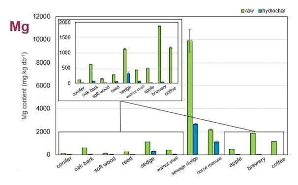
**Figure 32:** Balance of the Mg between the raw material (in green) and the hydrochar (in blue). To compare de value, hydrochar contents have been converted in mg.kg raw db<sup>-1</sup> according to equation **(10)**.
