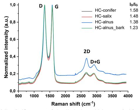
**Figure 23:** Normalised Raman spectra of selected hard carbons and their corresponding I<sub>D</sub>/I<sub>G</sub> ratios.
