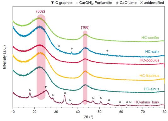
**Figure 22:** XRD patterns of the hard carbons from the different genera. Peaks are identified as:
