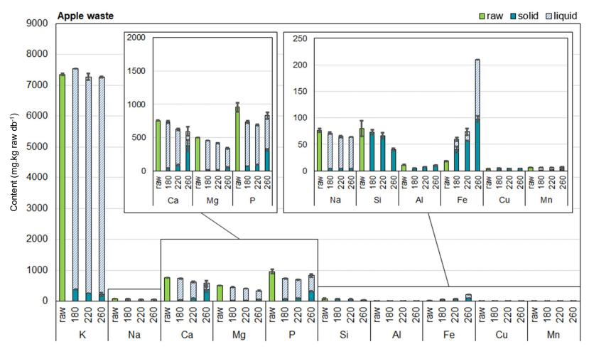
**Figure 60:** Balance of the inorganics between the raw material and the hydrochar (solid) and liquid at the different temperatures of 180, 220 and 260 °C from apple waste. The different elements were represented on different scale, depending on the content. The values were converted on mg of element per kg of raw biomass according to equations (10) and (11) for solids and liquids respectively in order to compare them together. Standard deviation are experimental between the replicates.
