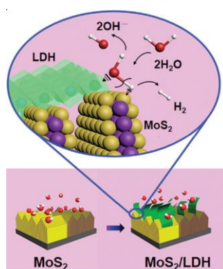
Figure 10: Schematic illustration of HER on MoS 2 /LDH in alkaline media showing the synergetic effect between LDH and MoS 2 . 26
