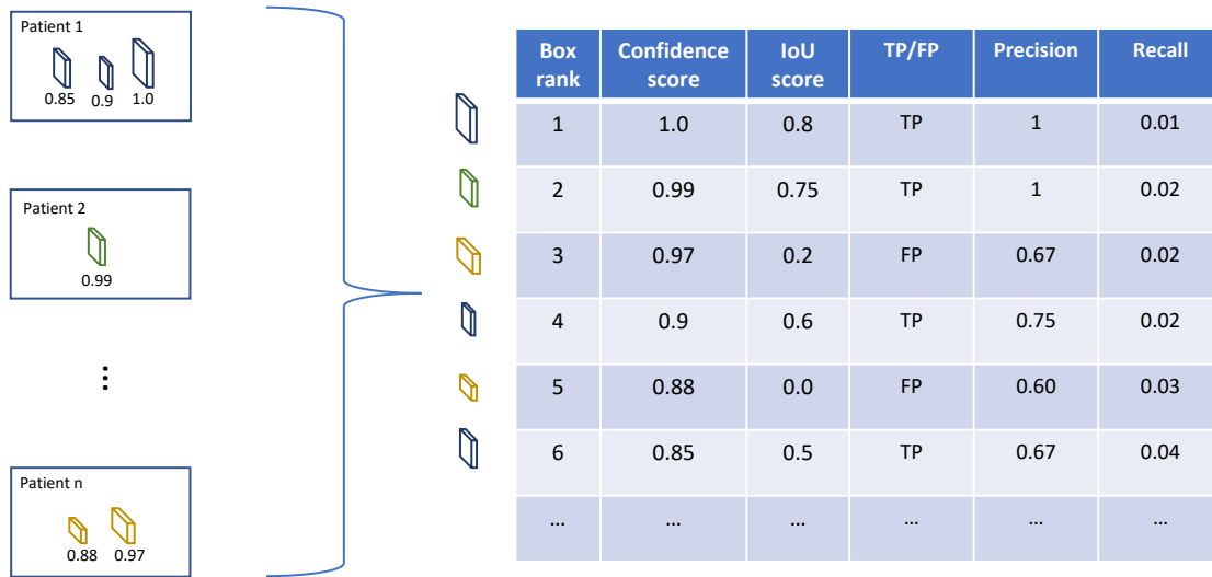
Figure 3.8: Workflow for computing precision and recall values in a context of nodule detection task, assuming IoU threshold \tau = 0.5 and the amount of nodule to detect is G = 100 .
