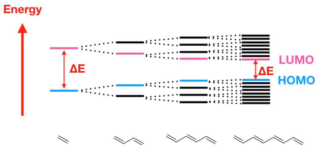
Figure 1.13. The energy gap between LUMO and HOMO.
