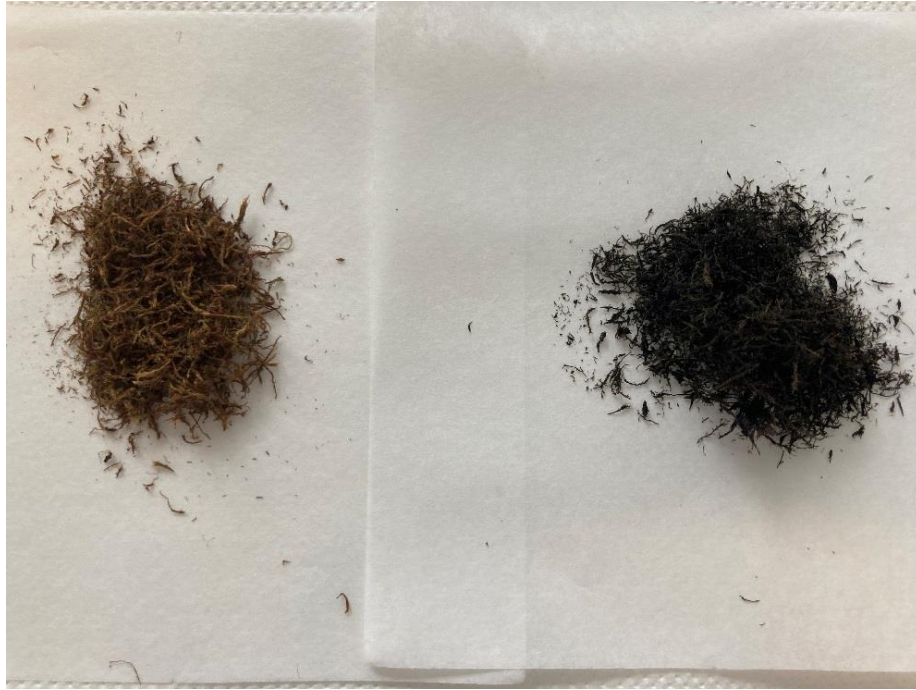
Figure 3.1. Photos of pristine GM (left) and GM-PMPG (right).
