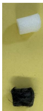
Figure 5.1. Photographs of the New Filter (upper) and the Filter-PetCoke composite (lower).
