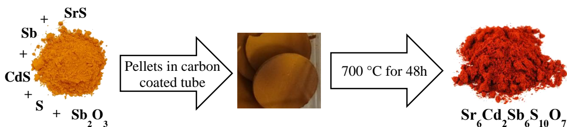
Figure 4.5 : Diagram of the solid-state synthesis of \text{Sr}_6\text{Cd}_2\text{Sb}_6\text{S}_{10}\text{O}_7
