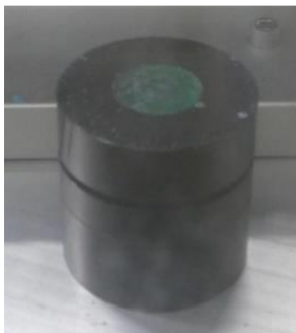
Figure 148 The sample holder designed Raman microscopy analysis of coated pellets
