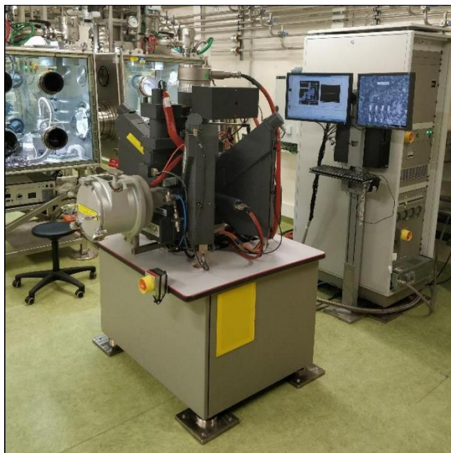
Figure 145 A photo of the CAMECA SX100 EPMA that is installed in the L26 laboratory in the Atalante facility
