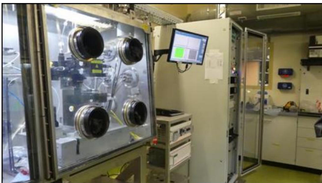
Figure 147 The Raman microscope installed in the L26 laboratories in the Atalante facility (the spectrometer on the right, the microscope inside the glovebox system)
