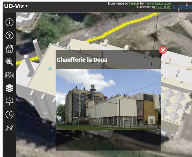
Figure 6.4.: The implemented nD urban data web application. The 3D scene contains a 3D model of the Chaufferie with a geospatial ‘pinned’ multimedia image of the factory overlaid using the technique proposed in [GDG22].
