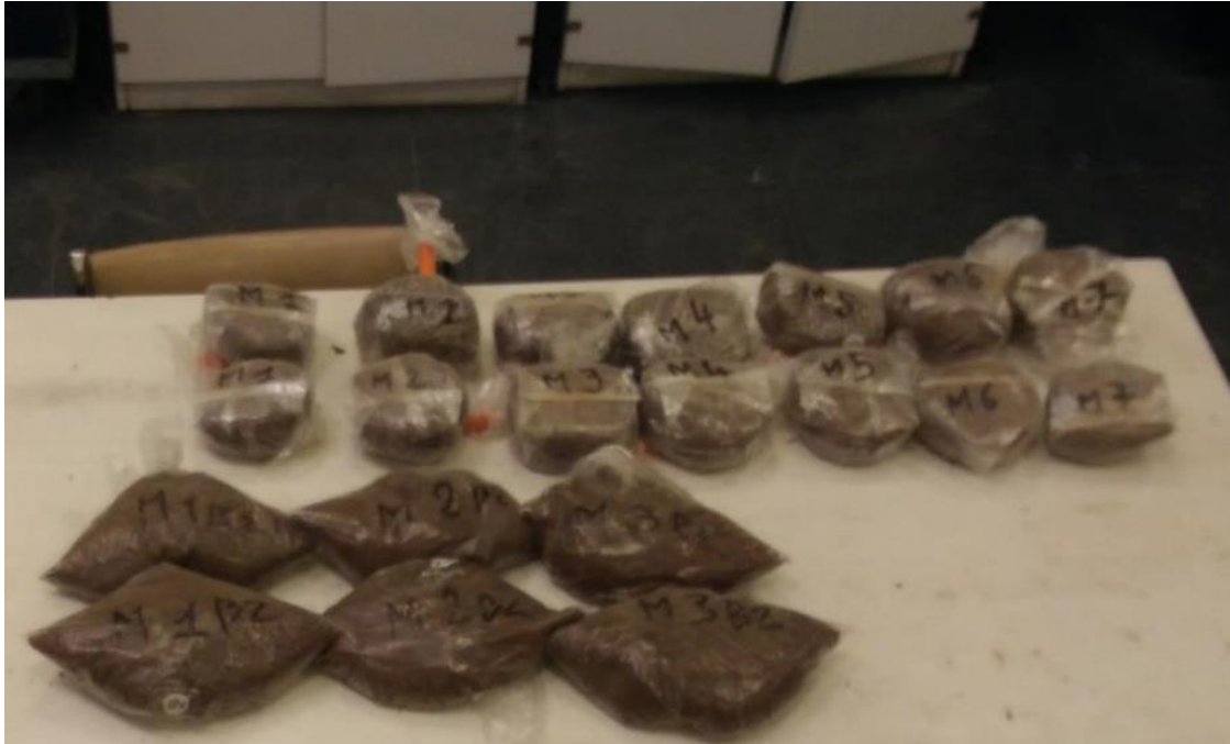
Figure 6.74: Picture, extracted from the test report showing the different specimens collected. On the top, 14 specimens of the wall for dry densities measuring. On the bottom, 6 earth bags for water content measuring
