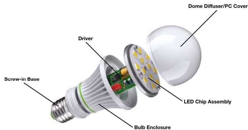
Figure 4.1: Taking apart an LED light bulb [92].
