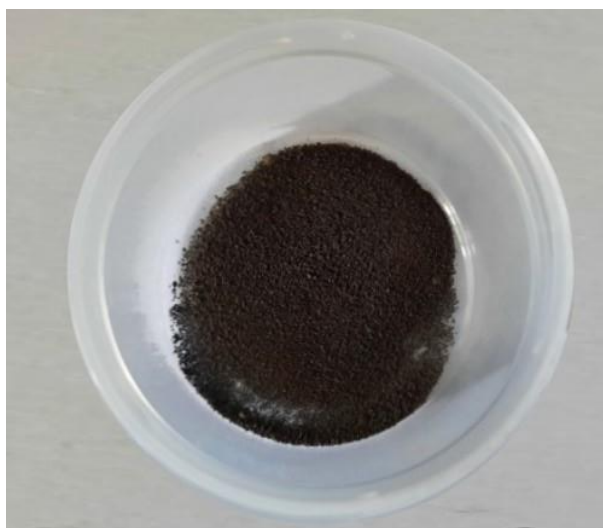
Figure 6.6 Resulting precipitate after one hour of formation at T = 25^{\circ}\text{C} , [\text{H}_3\text{PO}_4] = 25\% \text{P}_2\text{O}_5 , and Sulfur/ \text{Cd}^{2+} = 60/1 .
