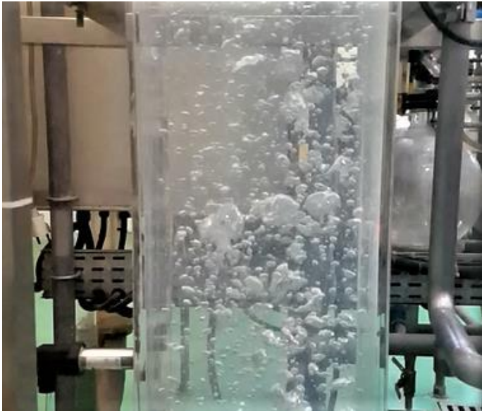
Figure 2.7 Example of bubbles using 30 ppm of ester, and U_g = 2.53 cm.s -1 .
