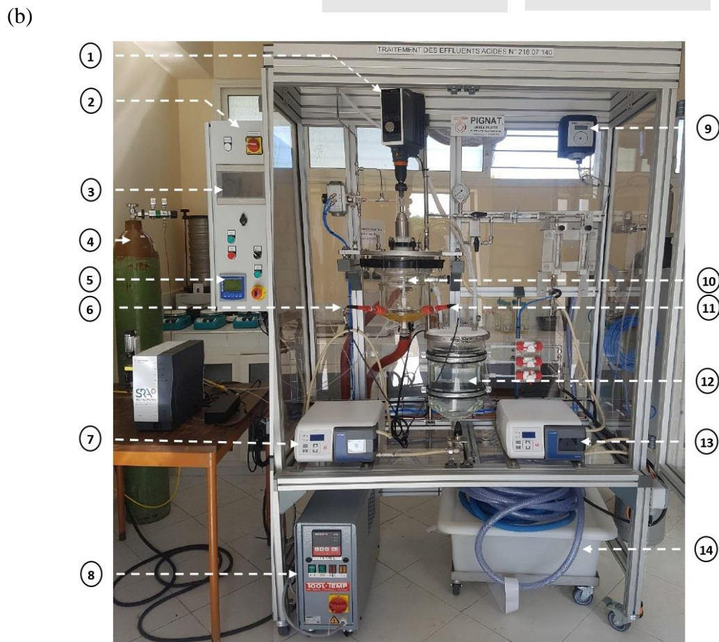
Figure 5.1 (a) Schematic and (b) photograph of the continuous pilot unit for cadmium sulfide precipitation from phosphoric acid effluent. ① Overhead stirrer, ② Electrical box IP55, ③ Touchscreen console, ④ Helium gas cylinder, ⑤ pH and ORP transmitter, ⑥ pH probe, ⑦ Peristaltic pump for H 3 PO 4 solutions, ⑧ Thermoregulator, ⑨ H 2 S gas detector, ⑩ Six blade Rushton turbine, ⑪ ORP probe, ⑫ Settler, ⑬ Peristaltic pump for sulfide solutions, ⑭ Tank for discharging treated effluent.
