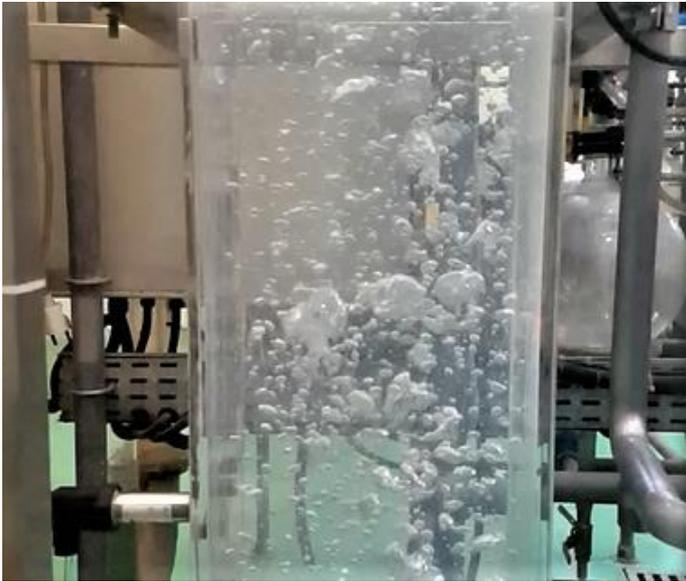
Figure 2.7 Example of bubbles using 30 ppm of ester, and  $U_g = 2.53$  cm.s<sup>-1</sup>.
