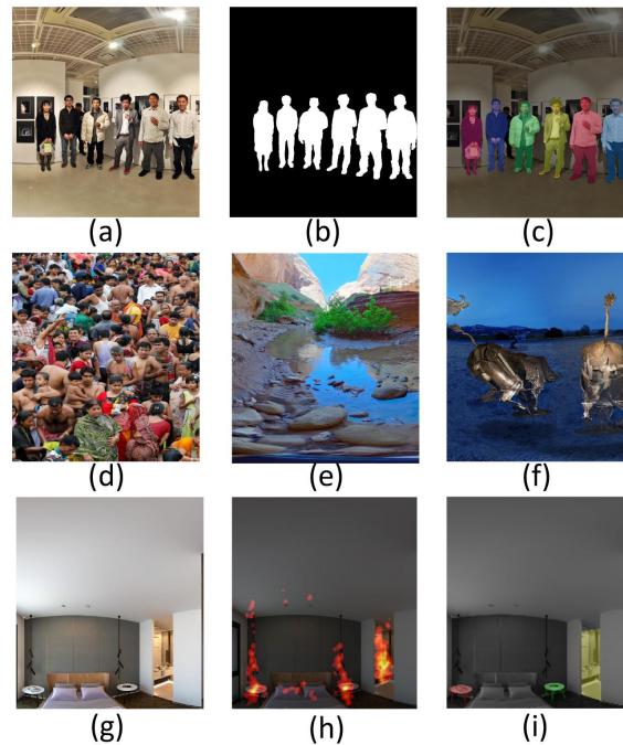
Fig. 3.1 A visualization example which illustrates partial key aspects of salient object segmentation construction. The first row indicates typical pixel-wise manual annotations in current salient object segmentation datasets, i.e. , object-level (binary) and instance-level masks. The second row shows specific real-life scenes (scattered people, pure background objects and meaningless foreground objects) tend not to be included in current most datasets. The third row shows salient objects defined with the guidance of fixations. This figure is cited from [281].
