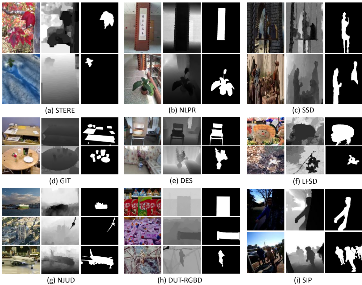
Fig. 2.9 An illustration of RGB-depth salient object segmentation. (a)-(i) are the examples of commonly used datasets for RGB-depth salient object segmentation. For each of the datasets, the ground truth, depth map and the given image are listed from right to left. This figure is cited from [208].
