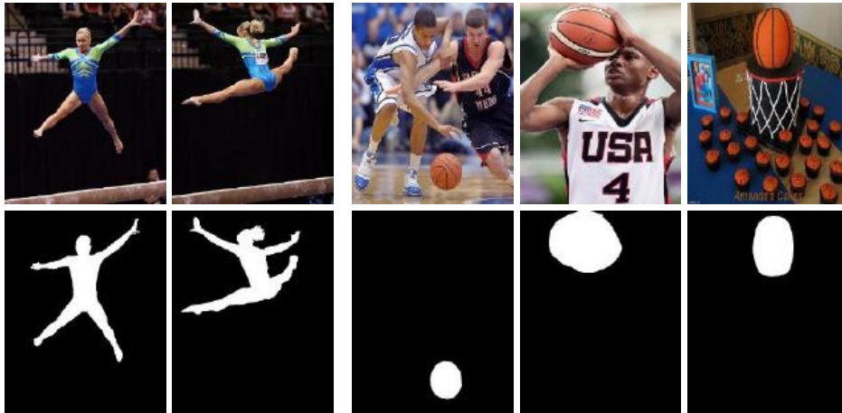
Fig. 2.7 An illustration of group(co)-salient object segmentation. There are two groups of images with specific classes of co-salient objects ( e.g. , gymnast and basketball), surrounded by similar or totally different background scenes. This figure is cited from [189].
