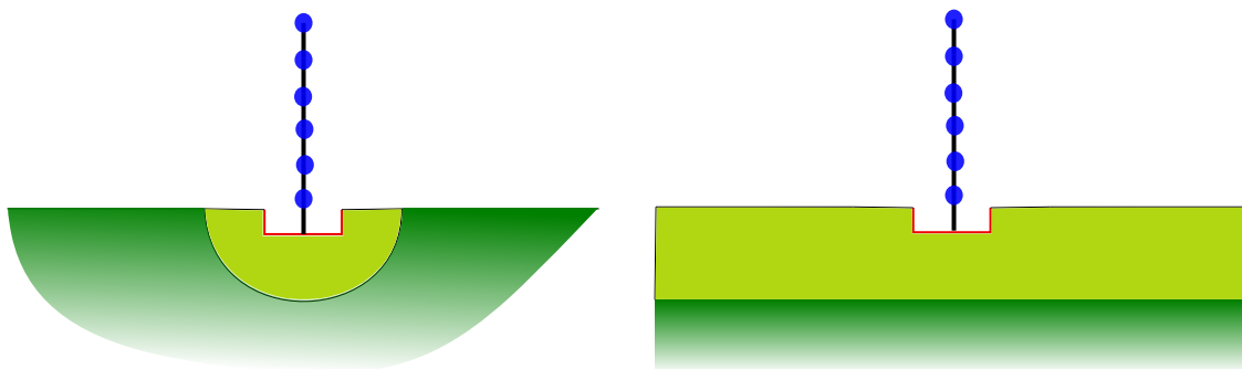
Figure 5.2.: Types of basin used: Case (a) hemispherical basin in homogeneous half-space (left) and Case (b) horizontally stratified basin (right).
