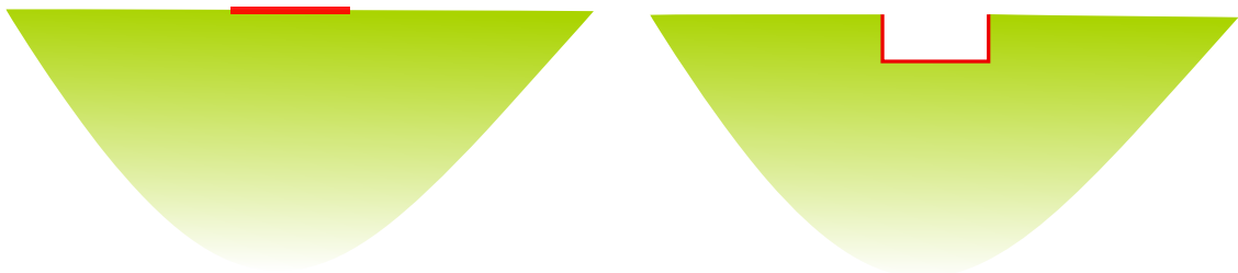
Figure 4.1.: Illustration of the two configurations considered for the validation of the impedance operator for a homogeneous half-space: surface (right) and embedded (left) footings.
