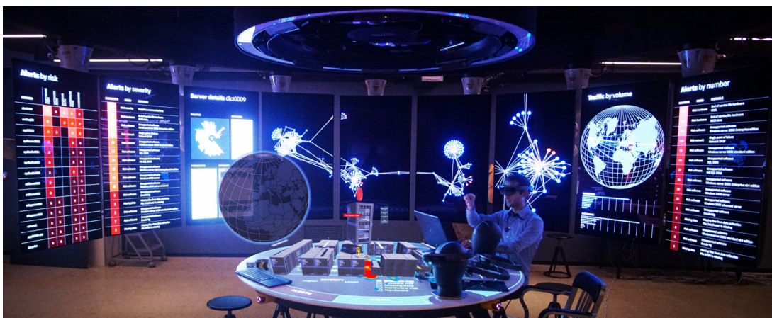
Figure 2.15 – DataSpace environment, with 15 high-resolution displays attached to robotic arms, 2 table projectors, AR and VR headsets; Cavallo et al. [158]
