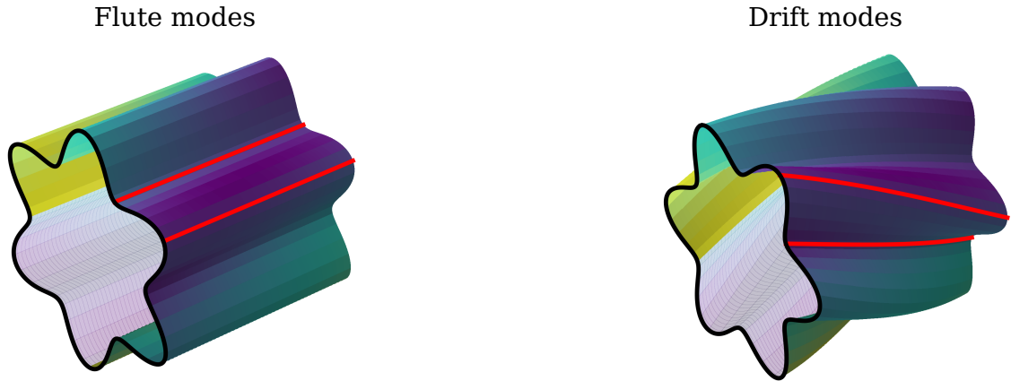
Figure 2.5: Flute (left) and drift (right) instability modes in a cylinder. Here, modes of m = 6 are represented with no parallel component to the magnetic field (i.e. n = 0 , flute modes) and with an arbitrary parallel mode (i.e. n \neq 0 , drift modes). Red lines are isocontours of the considered quantity, like pressure for example, and are twisted if n \neq 0 .
