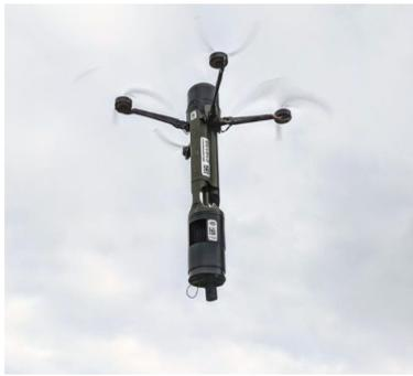
(b) Bomb-dropping UAV: De-fendtex d40
