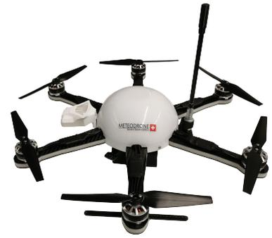
(c) Meteorology UAV: Meteorodrone MM-641/SSE
