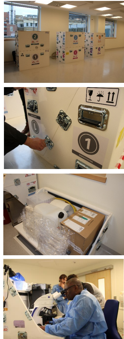
Figure 43: Photo taken during the MVP testing in February 2019. From top to down, all modules in closed position, opening of a module, Tetris like assembly in a module, module assembled, laboratory technician working on a module, Mini-Lab (France)
