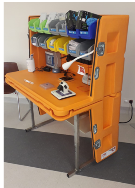
Figure 16: Photo of the Box-bench roto moulding pre-series test, Mini-Lab (France)
