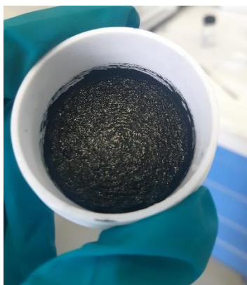
Figure IV-6. Slurry viscosity when using a) 10 wt. % of CMC-SBR (5-5) and b) 40 wt. % of CMC-SBR (10-30).
