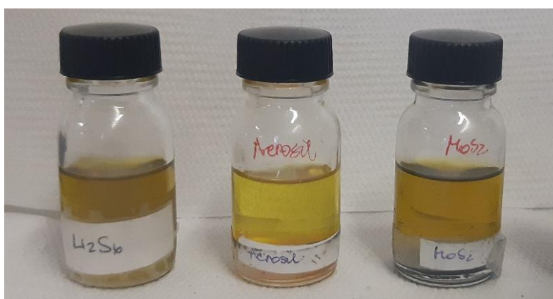
Figure III-32. Images of the 3 mM Li 2 S 6 color solution evolution after addition of Aerosil 200 and MoS 2 .
