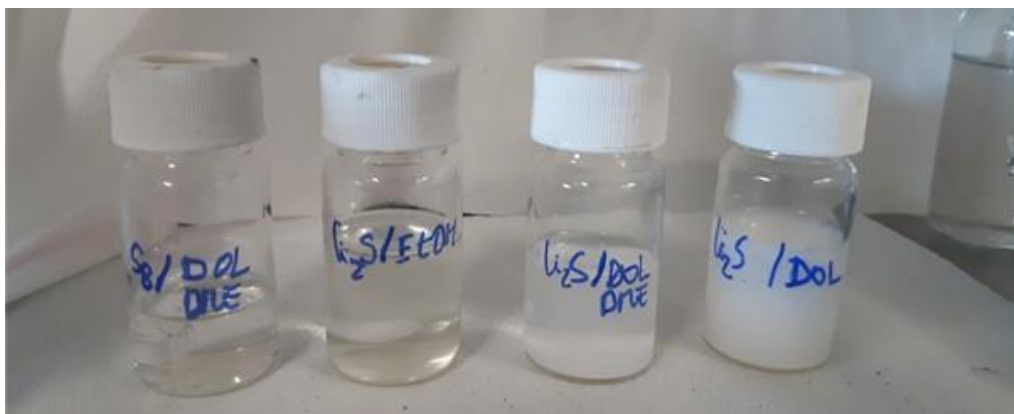
Figure III-1. Images of 0.4 mM S 8 in DOL:DME and 32 mM Li 2 S in different solvents.
