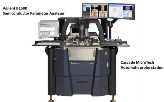
Figure 3.2 Agilent B1500 semiconductor parameter analyzer and 300 mm Cascade MicroTech probe station
